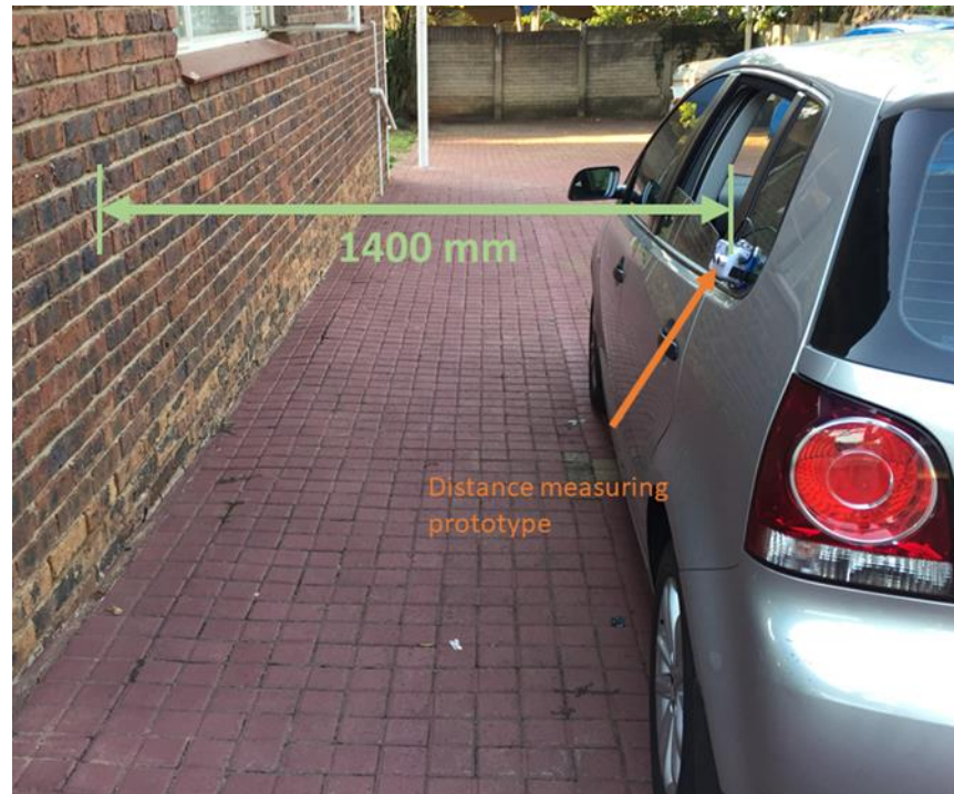
Figure 3-17: Experimental set-up depicting measurements recorded at a distance of 1400 mm
