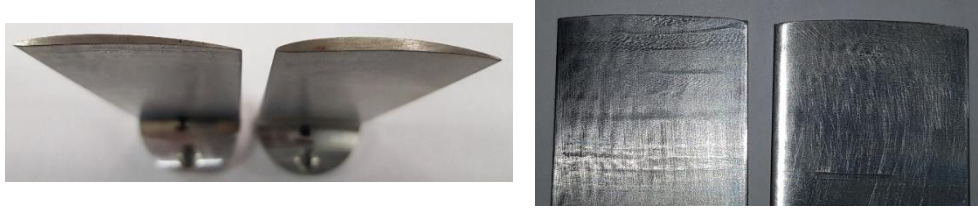
Figure 2.4. Manufactured blades showing the healthy and damaged blade (left) and the curved tips (right) to account for the casing curvature
