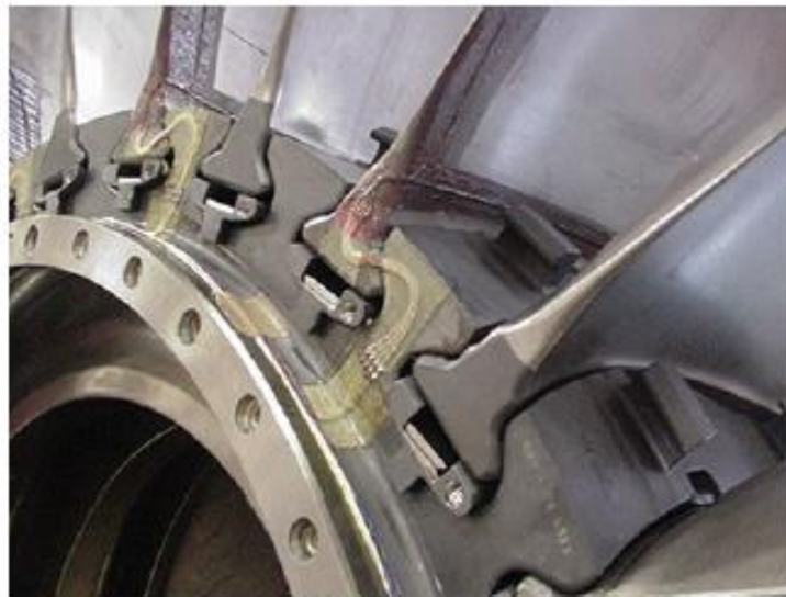
Figure 1.4. Typical rotor strain gauge installation (Adapted from Russhard, 2015)
