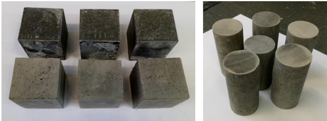
Figure 4-8: Cubes and cylinders used to obtain material strengths
