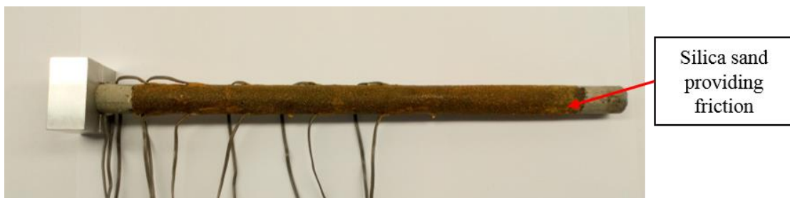
Figure 4-13: Instrumented scaled reinforced concrete pile – with silica sand
