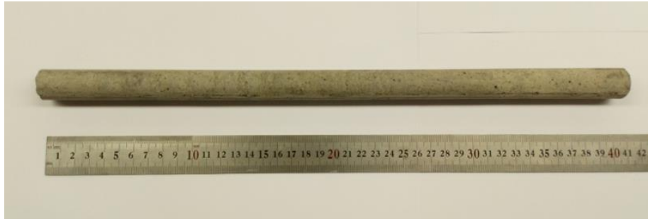
Figure 4-6: Completed model reinforced concrete pile
