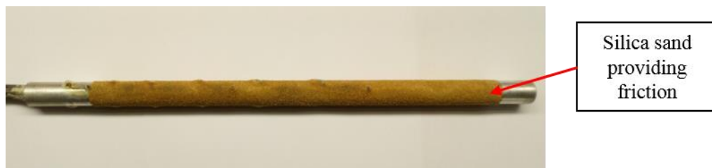
Figure 4-12: Instrumented scaled aluminium pile – with silica sand
