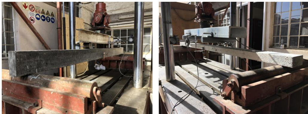
Figure 4-7: (a) 50 x 100 x 2000 mm beam and (b) 100 x 50 x 2000 mm test set-up
