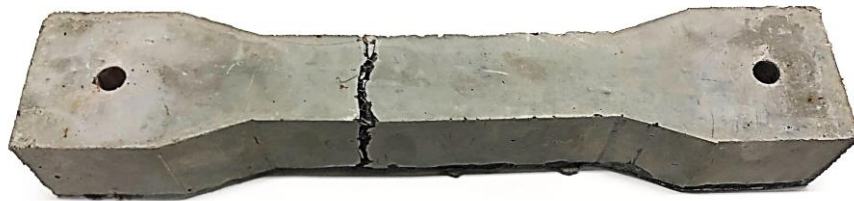
Figure 5-5: Dog bone specimen after test
