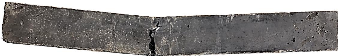
Figure 5-11: MOR beam after tested until failure
