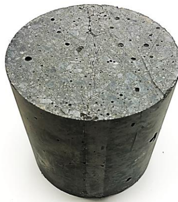
Figure 5-9: Split cylinder after tested until failure
