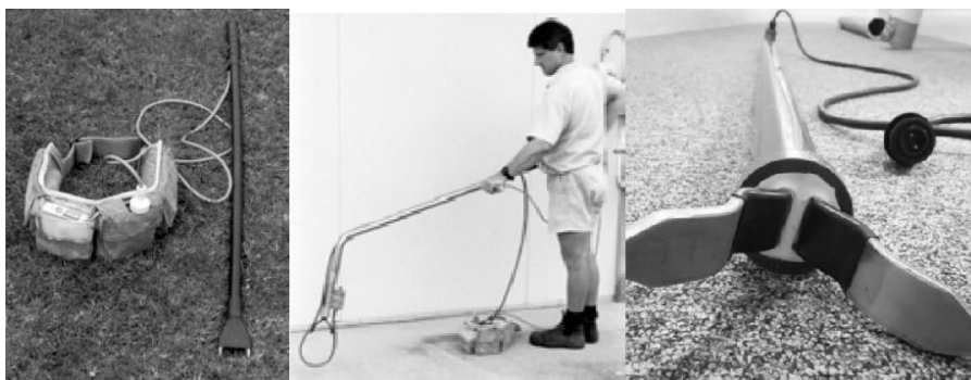
Figure 2.1: Electrodes of an e-stunner wand a) ballpoint pins, b) noose and fork-like wand and c) fork-like wand (Davis et al. , 2000; Livestock Welfare, 2017).
