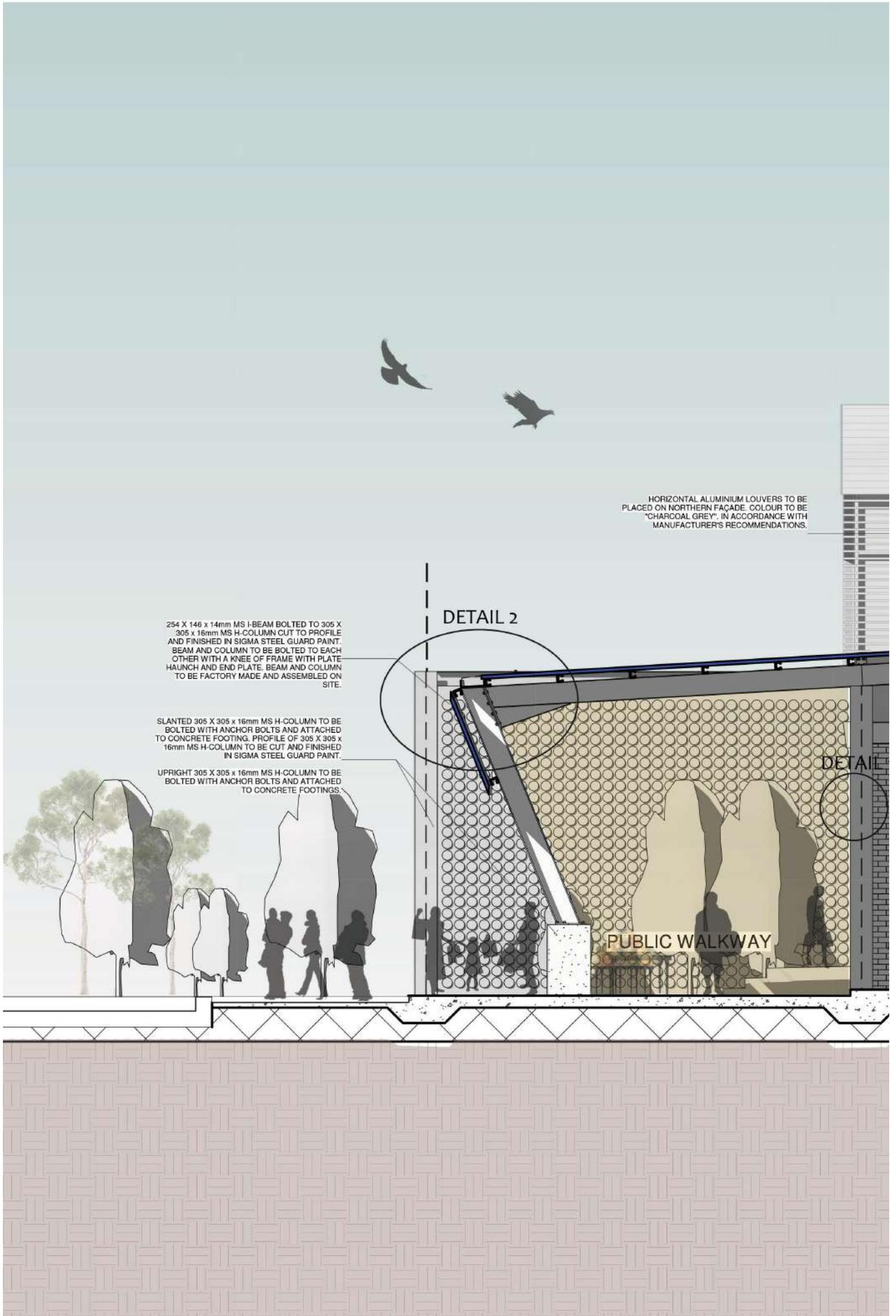
0.8MM CHROMADEK COLOUR BOND KLIPLOCK 700 SYSTEM, ROOF SHEETING WITH SISALATION FIXED WITH M8 BOLTED 100 75 X 20 X 3MM C-CHANNEL PURLINS, SPACED @ 1000 MAX C/C FIXED TO 254 X 146 X 14MM MS I-BEAM, COLOUR TO BE "CHARCOAL GREY", IN ACCORDANCE WITH MANUFACTURER'S RECOMMENDATIONS. SHEETING COLOUR - "CHARCOAL GREY". ALL EDGES, FLASHING, COUNTER FLASHING, GUTTERS, DOWN PIPES AND RAINWATER GOODS TO BE SAME COLOUR AS STEEL COLUMNS AND BEAMS - "CHARCOAL GREY"
