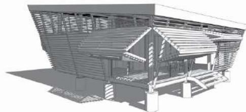
The structure is compiled of an inclined exterior façade which limits the amount of impact precipitation and sunlight has, thus limiting water splashing on the surface as well as overheating. The vertical structural columns carry of internal load therefore allowing the façade panels to be adaptable in order to regulate air flow through the building as well as to regulate views as desired (Ott 2019).
