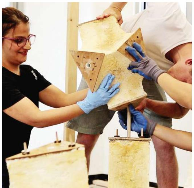
According to Hebel, there is great potential for mushroom mycelium to be used as structural elements for double storey buildings. Based on a 3D modelling program, templates of possible moulds were sent to a company called Mycotech in Indonesia that specialises in mushroom farming. Ultimately anyone who has access to a CNC machine can grow their own building structure based on a downloadable online design (Frearson 2019).
