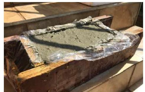
FIG 6.12: Making of crushed glass and concrete blocks (Made by Author 2019)
