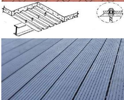
Composite deck system is used from the first floor upwards. Due to its non-slip, non-toxic, impact resistant and environmentally friendly nature, it is suitable for the interior and exterior application. Vertical ribs are bonded with concrete to for the composite flooring system (Simpson, 2014).
