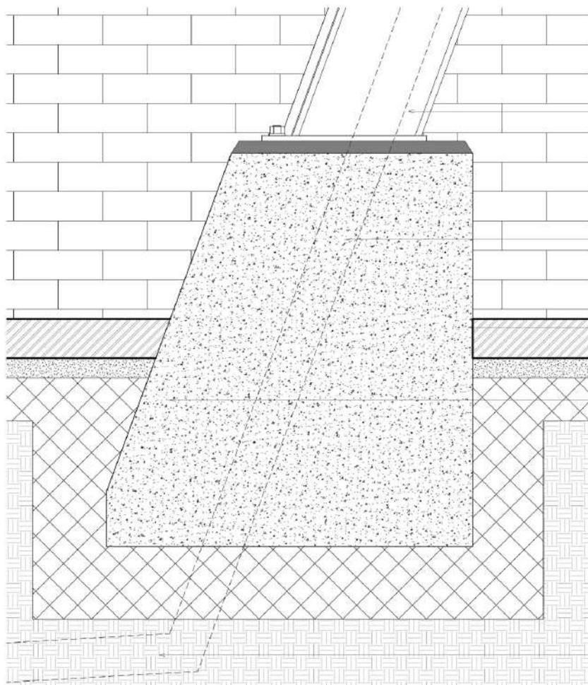
305 X 305 X 16MM MS H-COLUMN USED AS PRIMARY VERTICAL MEMBER. ALL COLUMNS AND BEAMS TO BE PAINTED WITH PRIMER AND FINISHED WITH SIGMA STEEL GUARD PAINT. BASE OF COLUMN TO BE BOLTED WITH ANCHOR BOLTS WITH BASE PLATE TO CONCRETE FOOTING AS PER ENGINEER'S SPECIFICATIONS.
