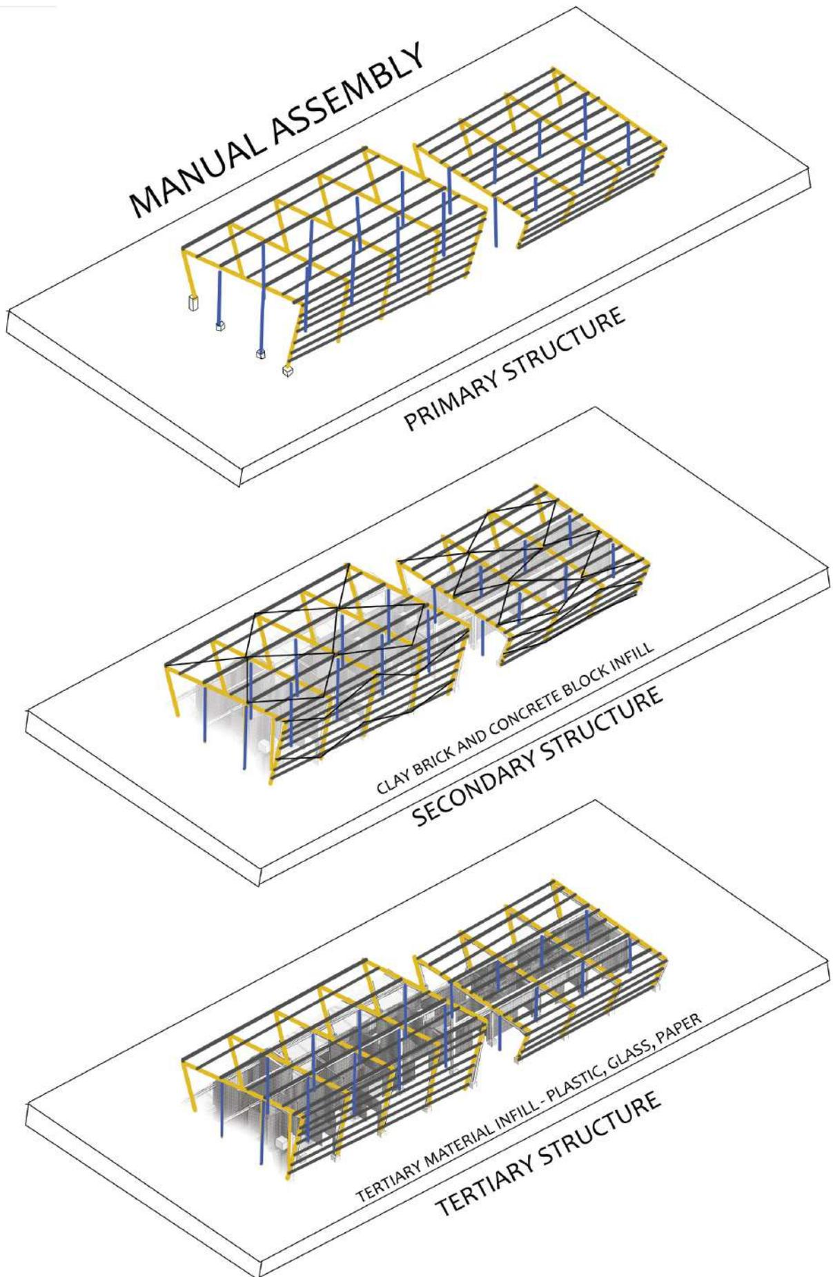
Fig. 7.7: Structure diagram demonstrating the primary, secondary and tertiary structure (Author 2019)
