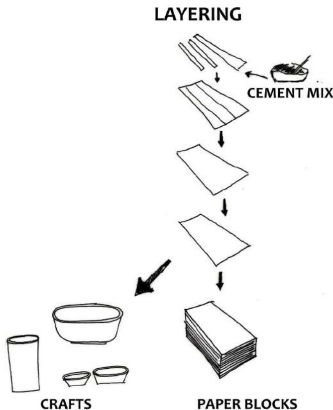
Fig. 6.6: The layering process of paper bricks (Author 2019)
