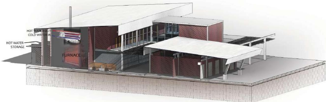
Fig. 7.15: Furnace and water heating sectional perspective (Author 2019)
