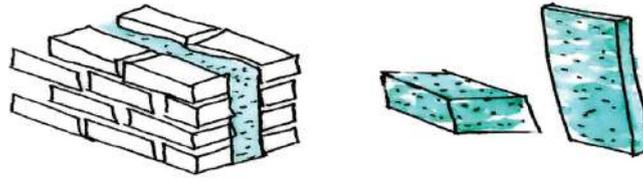
Mycelium components such as insulation and internal bricks
