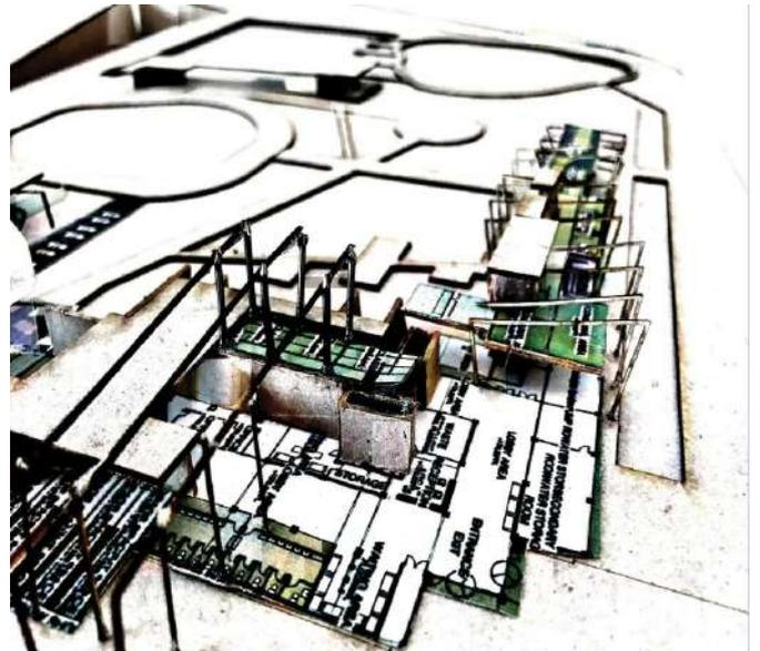
The breaking up of solid forms was the initial urban vision concept which allows for courtyard recreational areas as well as more green niches that are situated between masses. The span of the portal frames ranged to up to 12m span and therefore a steel column will be added at every 6m intervals in order to allow for manual assembly. This will enable future expansion to be easier.
