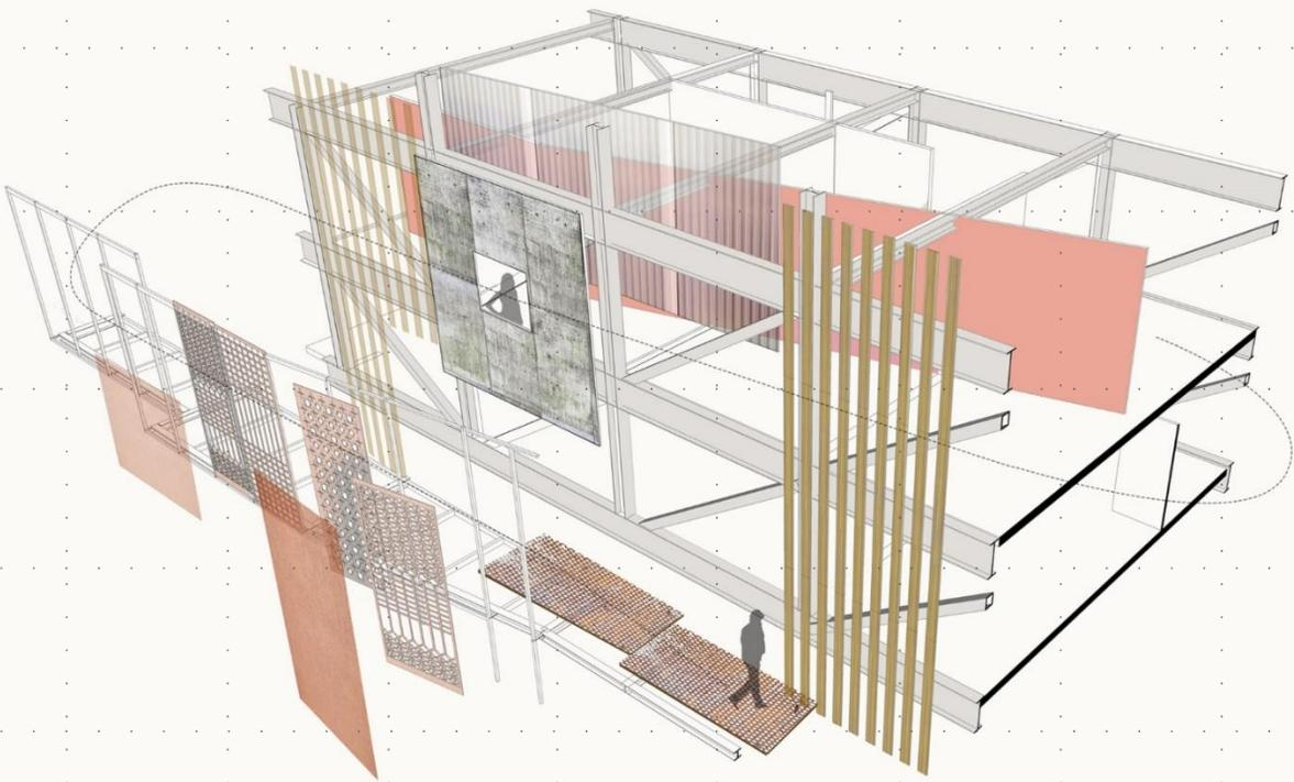
Figure 7.1 : Conceptual construction diagram expressing main structural systems and layering of materials . (Author:2019)
