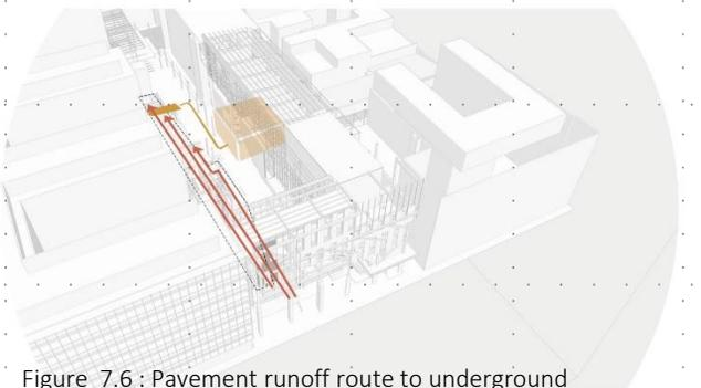
Figure 7.6 : Pavement runoff route to underground flush system and storage. (Author:2019)
