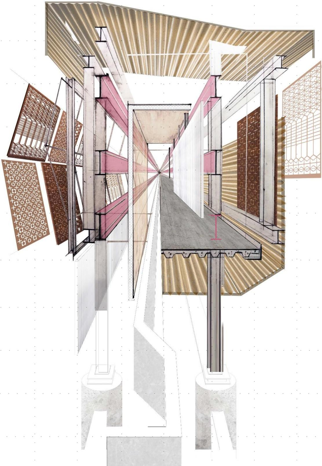
Figure 7.2 : Conceptual construction diagram expressing main structural systems and layering of materials . (Author:2019)
