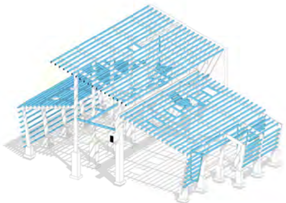
Figure 238: Secondary Structure (Author, 2019)
