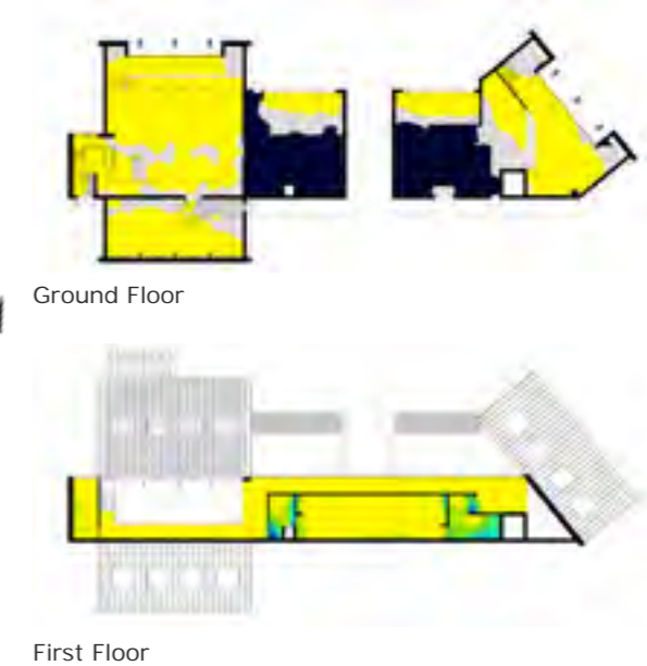
Figure 278: Iteration 3 - Over & Under-lit Floor Plans (Data Generated by Sefaria, Drawn by Author, 2019)
