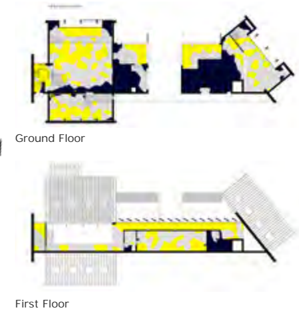
Figure 296: Iteration 6 - Over & Under-lit Floor Plans (Data Generated by Sefaria, Drawn by Author, 2019)
