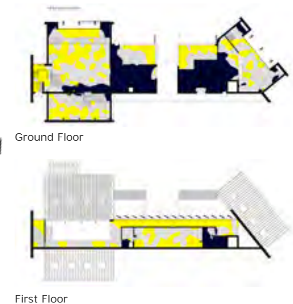
Figure 290: Iteration 5 - Over & Under-lit Floor Plans (Data Generated by Sefaria, Drawn by Author, 2019)
