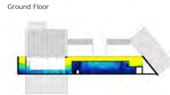
Figure 265: Iteration 1 - Daylight Factor Floor Plans (Data Generated by Sefaria, Drawn by Author, 2019)
