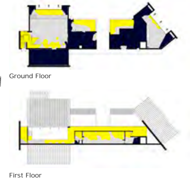
Figure 272: Iteration 2 - Over & Underlit Floor Plans (Data Generated by Sefaria, Drawn by Author, 2019)
