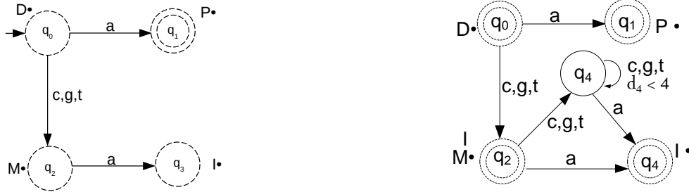
(a) A mono- pCA_{T_3} where at most 1 insertion is allowed before a perfect match.
