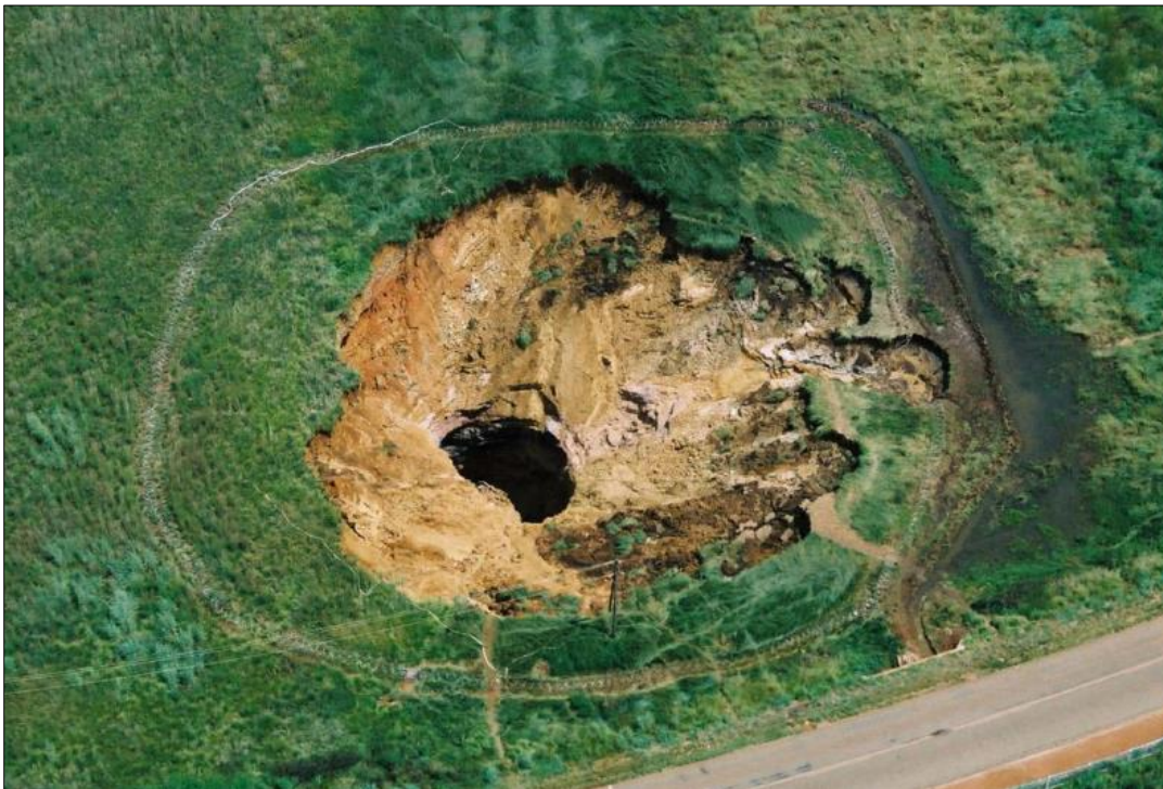
Figure 2-4: Aerial image of a sinkhole formation near Bapsfontein, Gauteng (Oosthuizen & Richardson, 2011)
