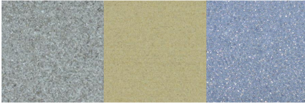
Figure 3-8: Materials tested in the centrifuge: (a) coarse-grained sand (Consol), (b) fine-grained sand (Afrimat) and (c) glass beads
