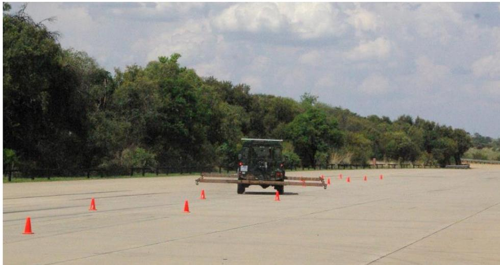
**Figure 53 Vehicle Exiting ISO3888-1 Manoeuvre, Note Brake Lights**
