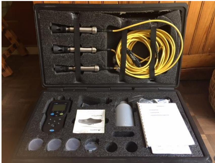
*Fig. 3-2 HACH® HQd IntelliCAL Rugged field kit*
