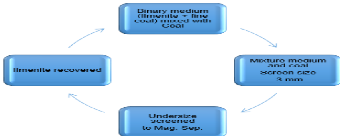
Figure 24 Reused ilmenite medium circuit
