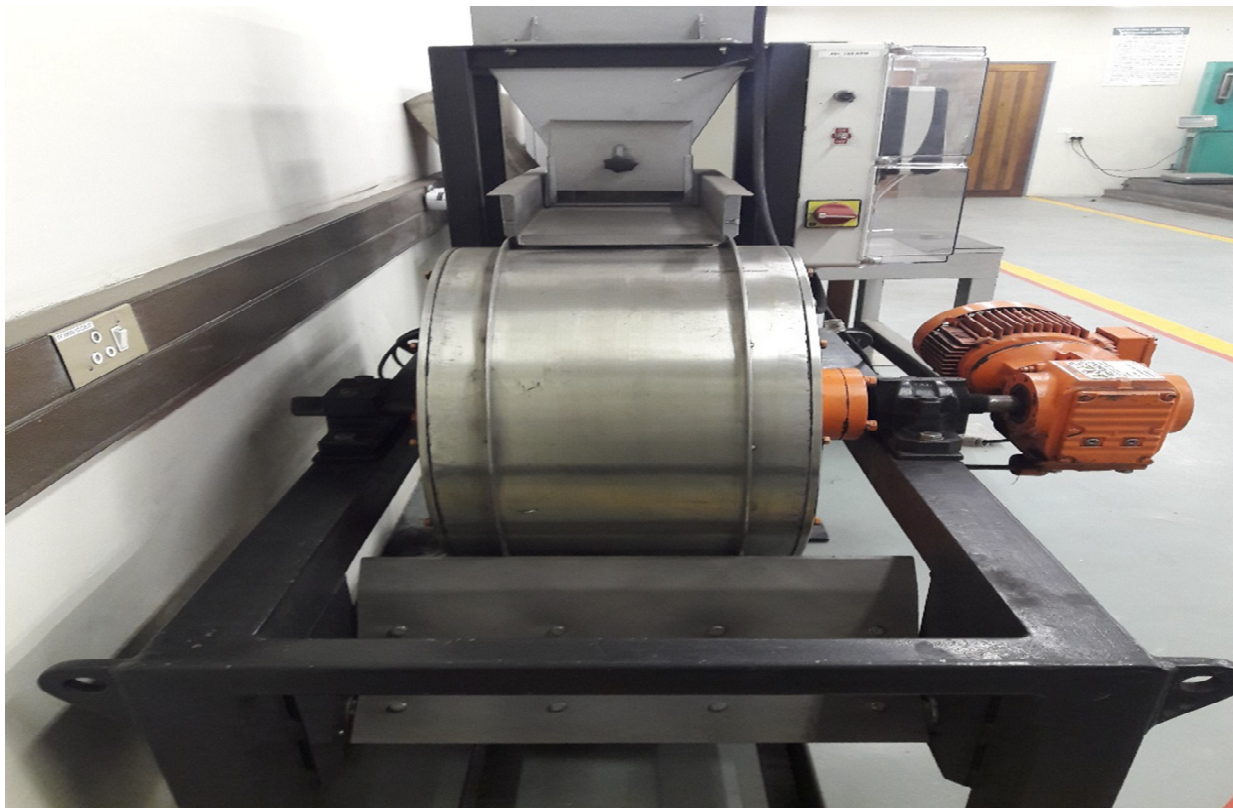
Figure 25 High gradient magnetic separator
