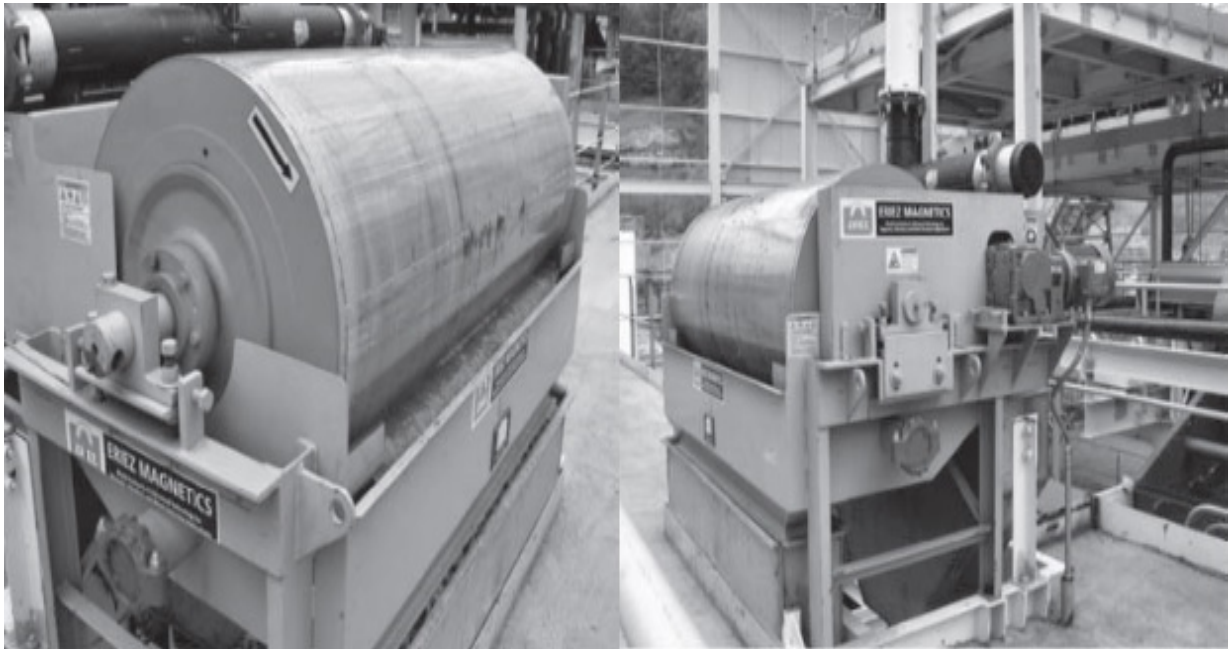
Figure 10 Wet drum magnetic separators for heavy media application. Self-levelling counter-rotation tank style (Norrgran, 2010).
