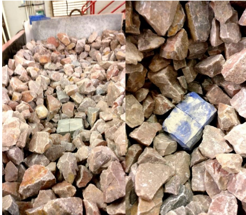
Figure 4-1: Kli-Pi 2 and 1 positioned at depths of 100 mm (left) and 250 mm (right) in the ballast box
