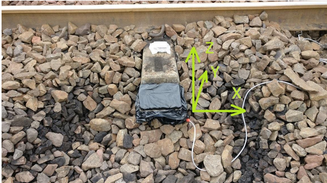
Figure 4-4: Wi-Fi AP with both the Ethernet cable and Kli-Pi 4 visible
