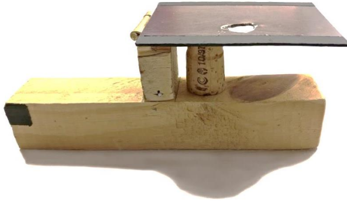
Figure A-2: Calibration tool assembly with a rotating platform about the hinge
