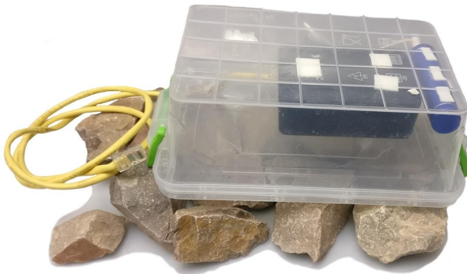
Figure 3-7: Raspberry Pi access point with visible Ethernet cable and a rechargeable USB power supply
