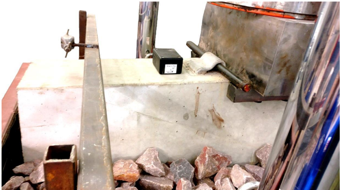
Figure 3-9: Box test configuration with the IMU (center) and the LDVT (left, not shown) bracket
