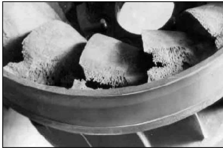
Figure 2-37: Cavitation Damage on Francis Turbine Runner (Brennen, 1994).
