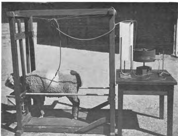
Photo No. 7.—Improved apparatus for recording ruminal movement. Water manometer method.
