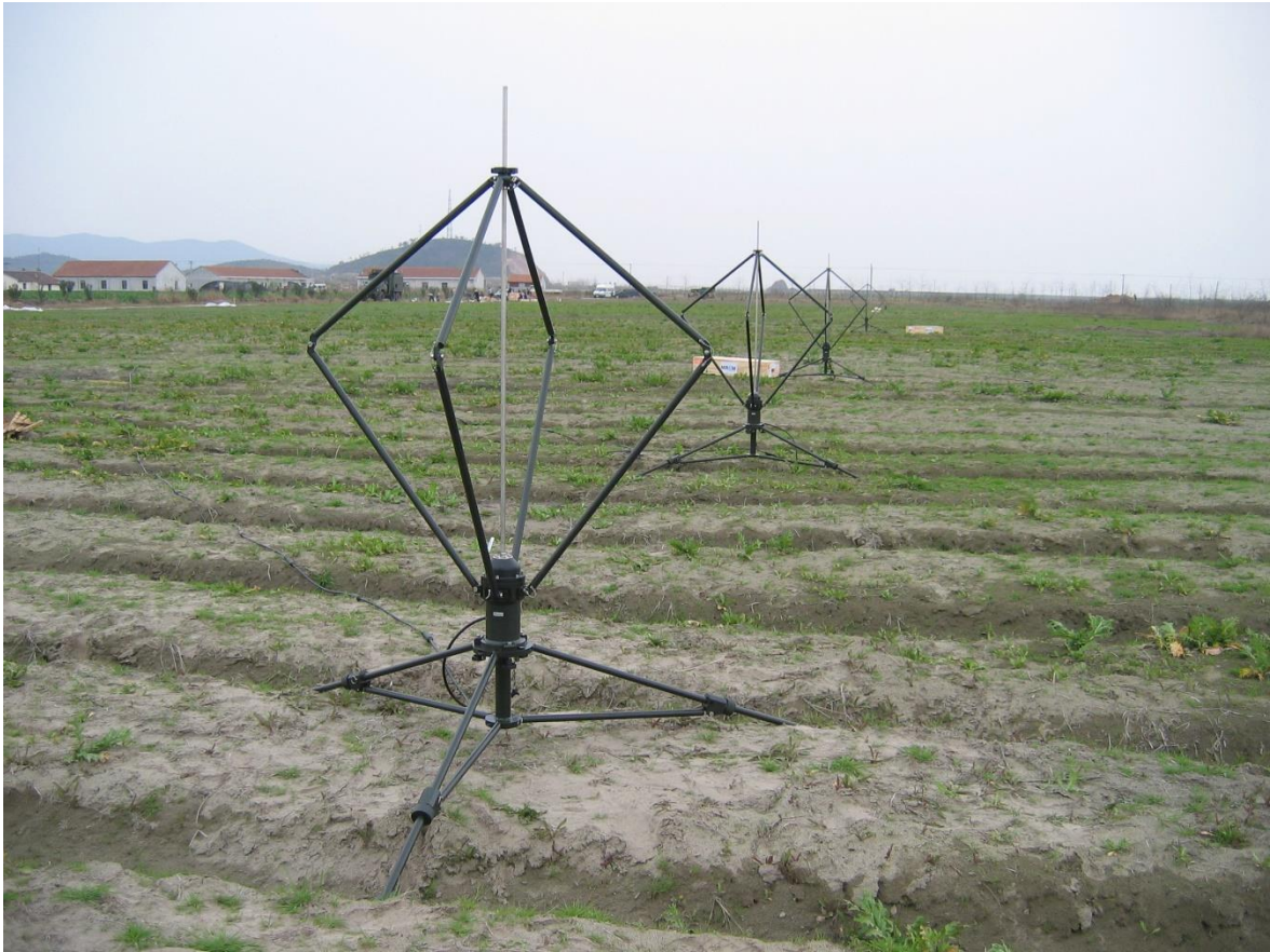
Figure 4.10. A photo illustrating the deployed antenna array utilised by the GEW MRD5000 wideband interferometric DF.
