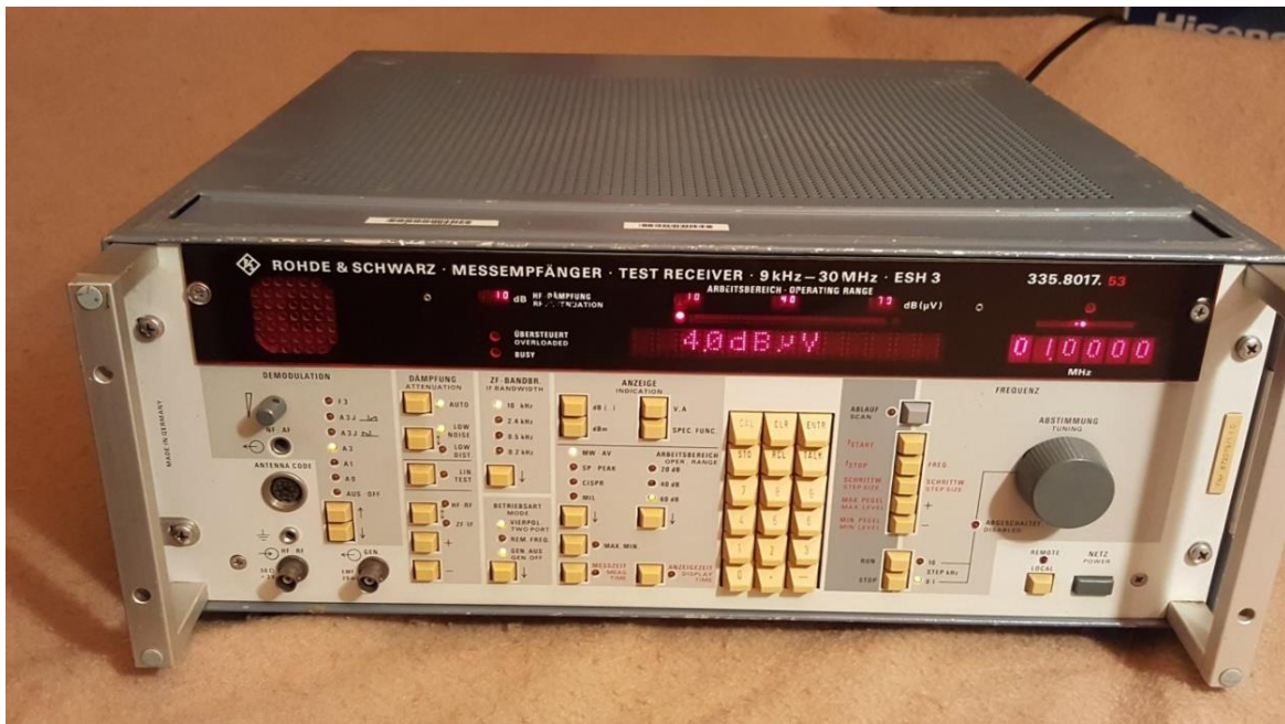
Figure 3.3. Rohde & Schwarz ESH 3 test receiver.
