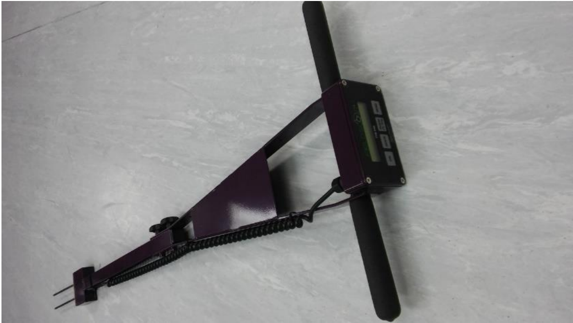
Figure 2.2. Example of the Fieldscout TDR 300 soil moisture meter (Spectrum Technologies, IL, USA).
