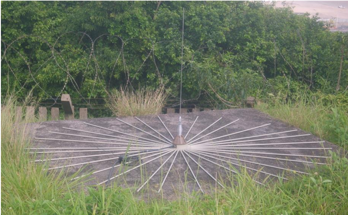
Figure 3.2. Example of an antenna used for field strength measurements.
