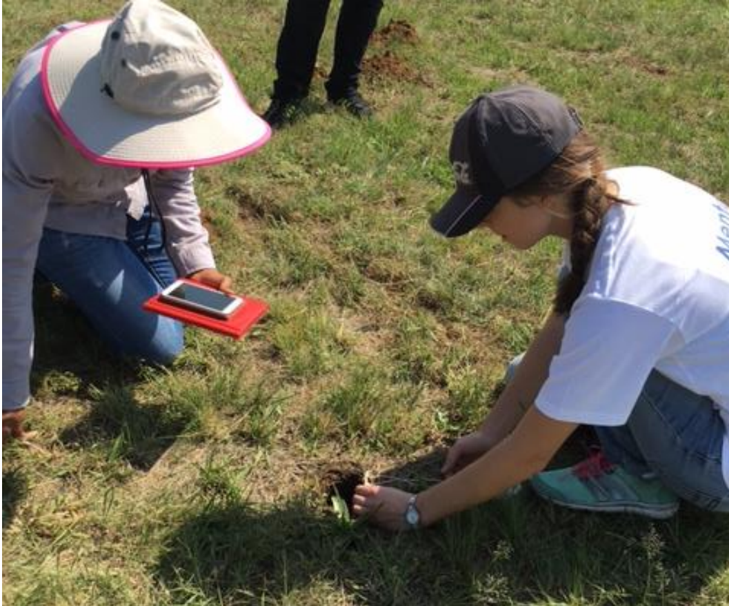
Figure 13: Sarah Mahlangu and Chantelle Schmidt conducting a percolation test in one of the augured holes at the study site.
