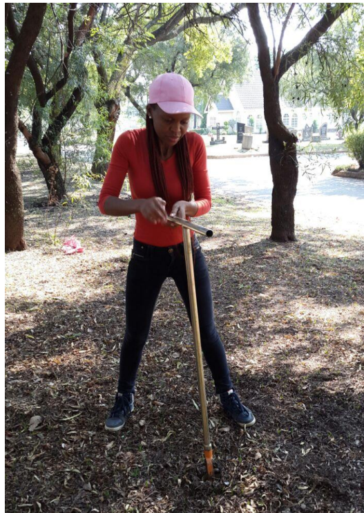
Figure 11: Hand Auger drilling at Fontein Street Cemetery.
