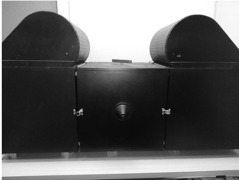
Figure 3.9 Front view of assembled test setup. This shows the side booths on both sides of the rotating mirror section. The eye piece is in the centre of the mirror section and the rotating mirror lever can be seen on top.
