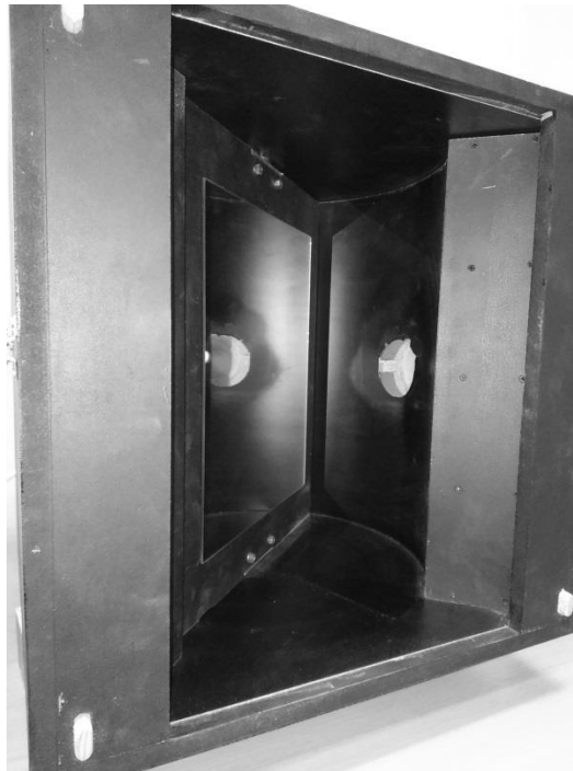
Figure 3.11 Rotating mirror section. The rotating mirror can be seen on left and eye piece entrance is visible on the left.
