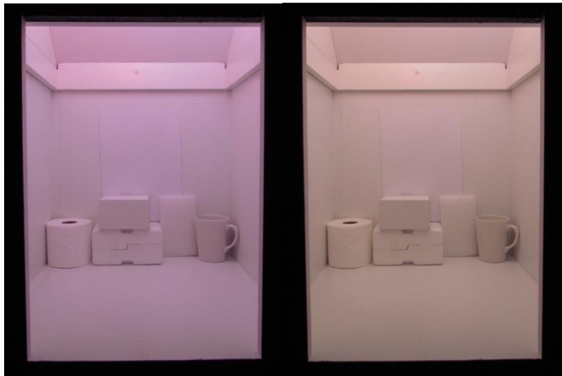
Figure D1. Test booth on the left is illuminated by a source selected by the under-40 group as yielding “white” light. It shows a higher component of blue. The test booth on the right is illuminated by a source selected by the over-50 group as yielding “white” light. It shows a smaller component of blue and a larger component of yellow.
