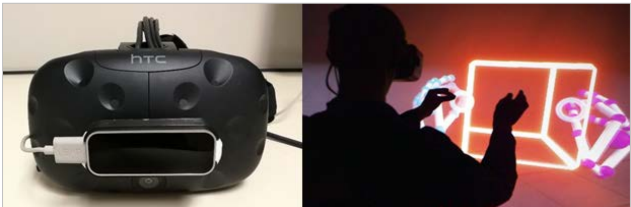
Figure 32: The HMD-mounted Leap Motion that was used (left) which allows a user to use their hands to interact with virtual objects in front of them (right) (Lang 2016)
