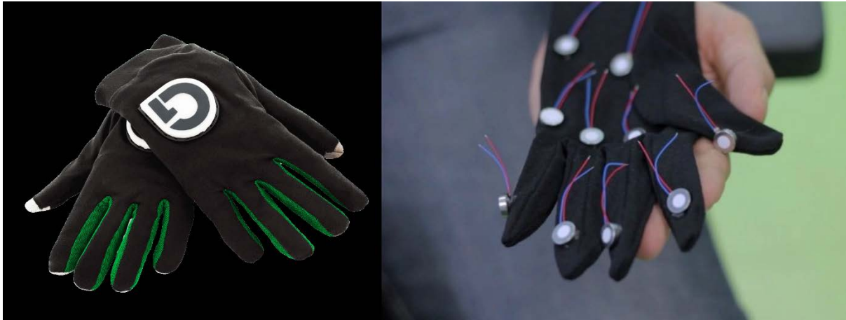
Figure 22: The GloveOne (NeuroDigital Technologies n.d.) uses vibrotactile actuators (right) to create various cutaneous sensations (Hayden 2015)
