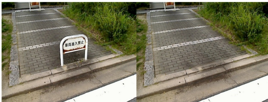
Figure 6: Diminished reality systems can “remove” objects from the world by supplying the user with a modified video feed where an object has been replaced with appropriate background textures in real time (Kawai, Sato & Yokoya 2016:1)
