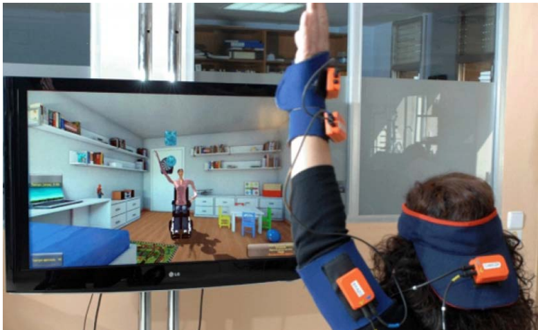
Figure 13: This VR telerehabilitation system lets users perform rehabilitative tasks at home while collecting data about their treatment (E-Health Reporter 2013)
