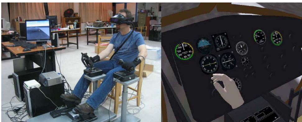
Figure 16: A virtual reality system (left) that lets users fly a virtual helicopter (right) by interacting with a virtual cockpit (Yavrucuk, Kubali & Tarimci 2011:3, 5)
