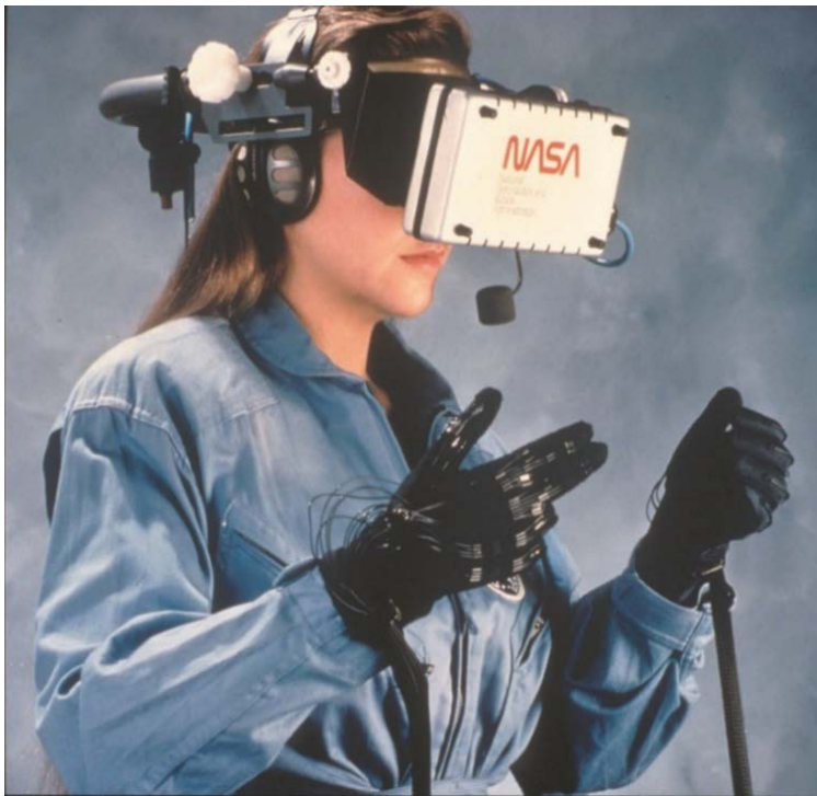
Figure 10: This image from 1990 shows someone using the virtual interface environment workstation (VIEW), which included head-, hand- and body-tracking (Rosson 2014)
