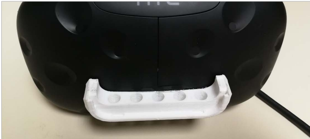
Figure 33: The modified version of the official Leap Motion VR Developer Mount that was used
