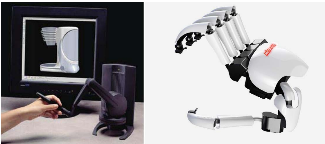
Figure 21: The PHANTOM Desktop (left) can prevent users from pushing forward (Berkley, Kim & Hong 2012:1) while the Dexmo (right) provides individual force-feedback for each finger (Dexta Robotics 2016)
