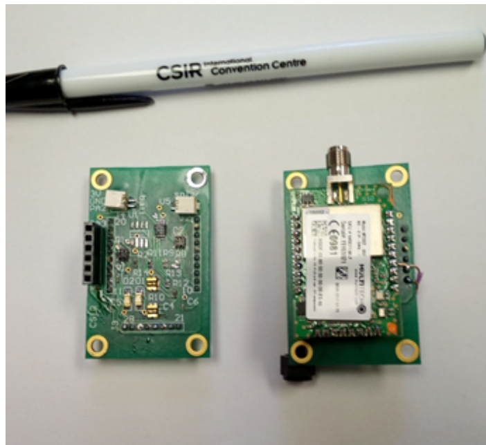
Figure 3.3. The PCB developed for the testbed.
