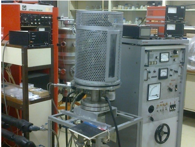
Fig. 4.3 A picture of the resistive evaporation system used to deposit Schottky contacts.
