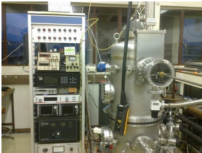
Fig. 4.2 A picture of the electron beam system used for ohmic contact deposition.
