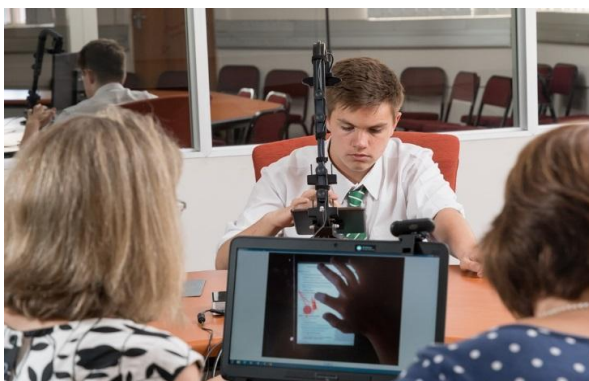
Figure v: Tobii mobile device stand with scene camera and Tobii X120 eye tracker
