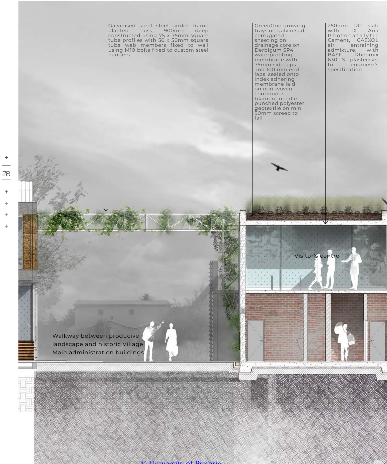
Fig. 7.55: Portion of section 1 (Scale 1:100, original drawing 1:50)(Author:2018)
