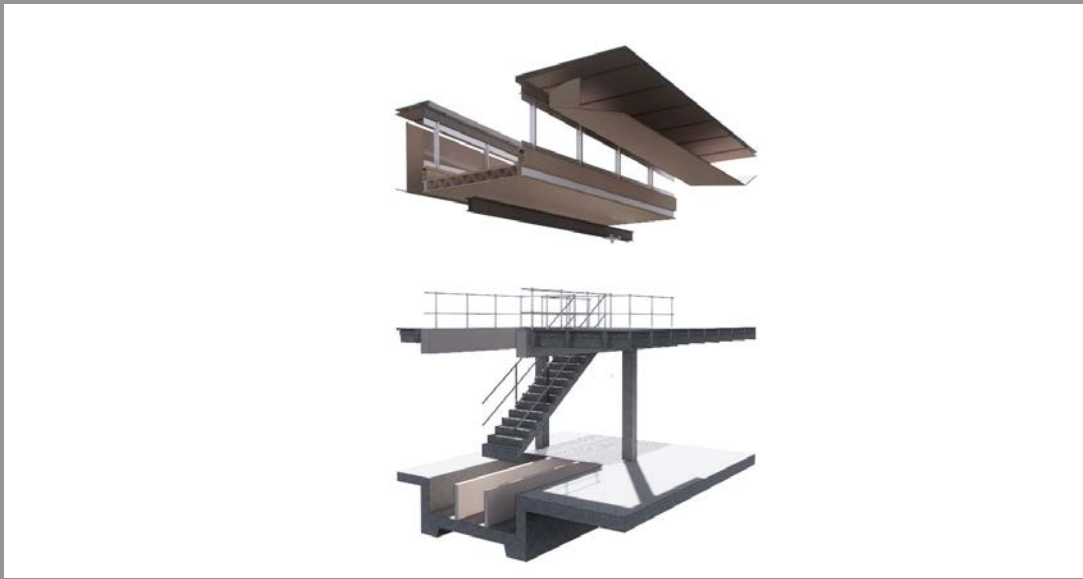
Fig. 7.26: Production space: planted roof and service channel in floor (Author:2018)
