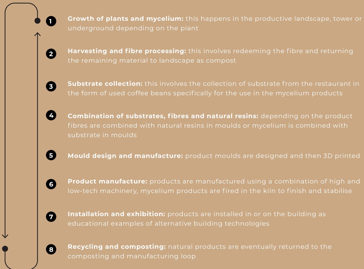
Fig. 7.22: Closed-loop bio-composite production process (Author:2018) (Based on Ecovative in SBIR (2015))
