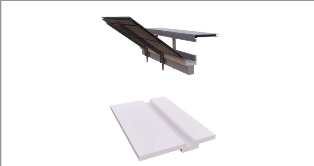
Fig. 7.27: Design space: roof water collection and floor service channel (Author:2018)
