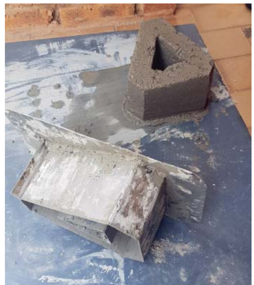
Figure 6.111 Block mould making and the casting of concrete (Author 2018).
