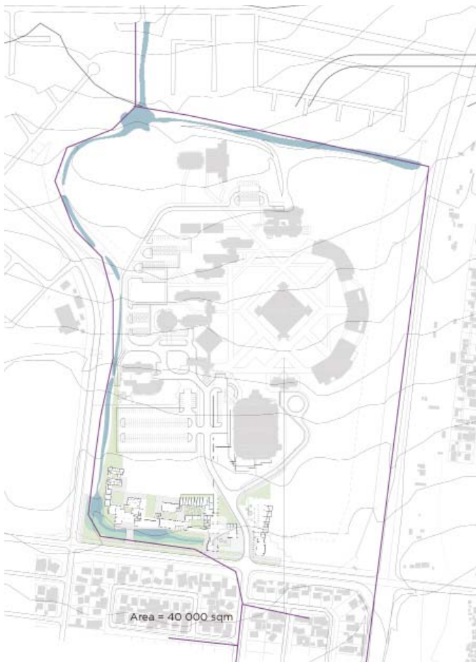
Figure 6.116 Left: Local storm water control and position of the storm water landscape (bioswale in relation to the rest of the regional storm water system). (Author 2018).
