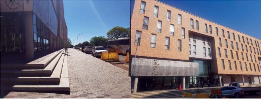
Figure 3.58 Sol Plaatje University (Activate Architects). The edge condition to the public square wraps around the corner and continues along the street edge. Level differences are negotiated using steps, which become seating in the shade of the building. Wheelchair accessibility is achieved as the levels merge in the square (Author 2018).
