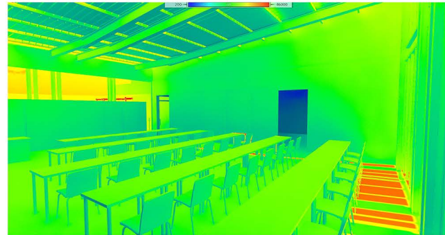
THIRD ITERATION ENTIRE FACADE CHANGED TO DANPALON, BETTER SPREAD OF LIGHT IN ROOM, BACK ROW OVEREXPOSED.
