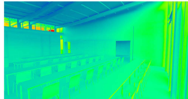
FOURTH ITERATION SHADING-DEVICE OUTSIDE ITERATED TO GET BEST POSSIBLE SPREAD OF LIGHT AND STOP OVER EXPOSURE IN THE ROOM.
