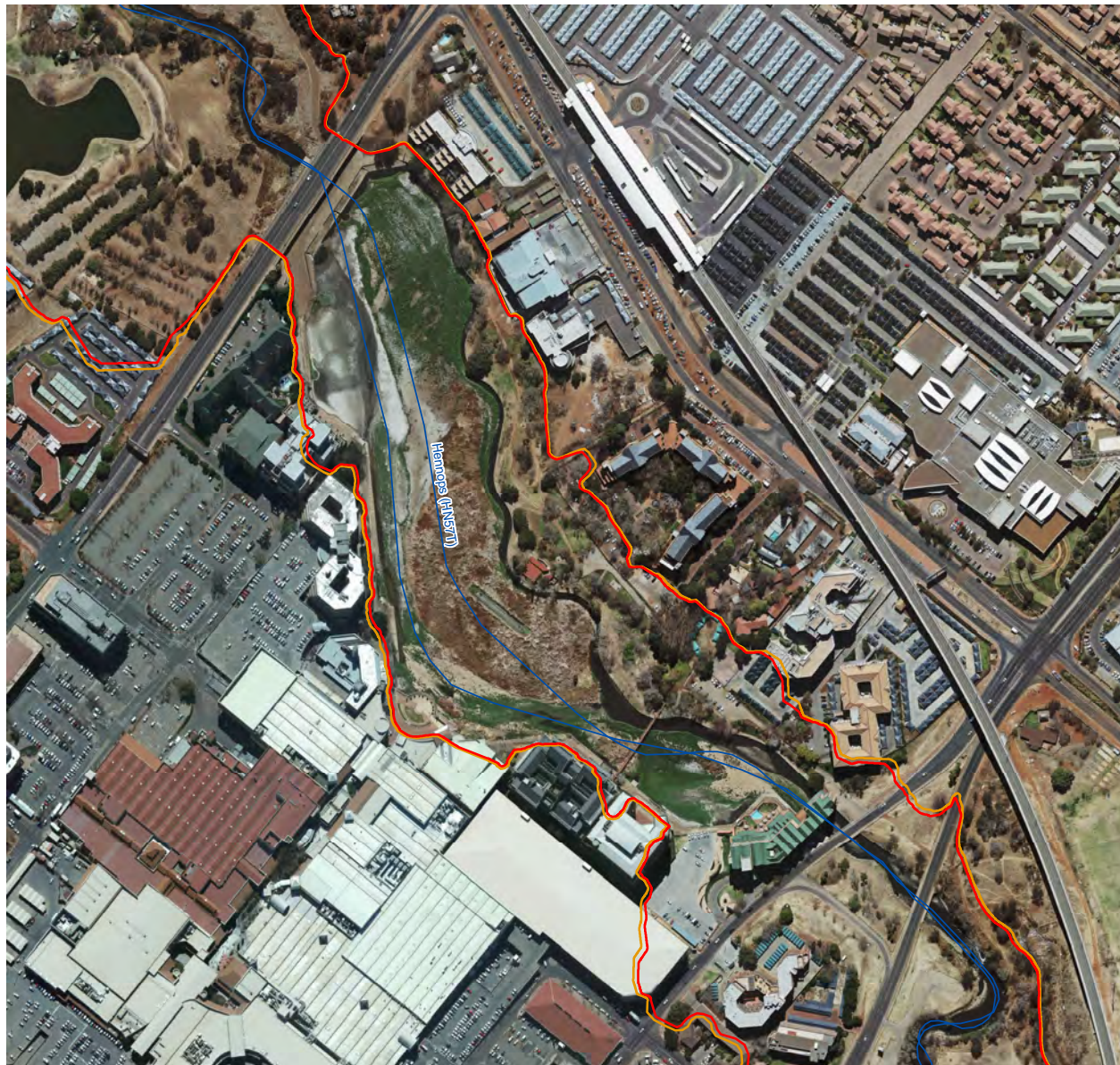
Figure 3.73 - Image highlighting two flood line scenarios; the red line indicates the 50-year flood line and the orange line marks the 100-year flood line (Tshwane Municipality, 2018).
