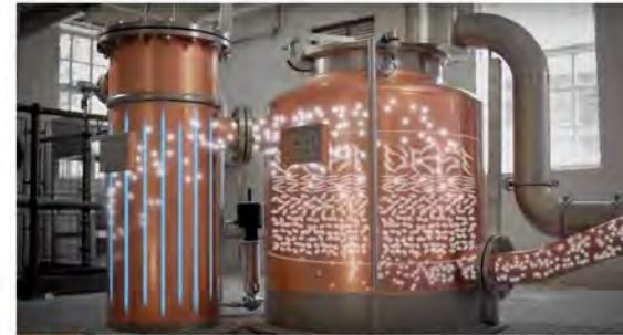
4 Vapour Infuser and Condenser: Vapour Infusion and condensation processes
