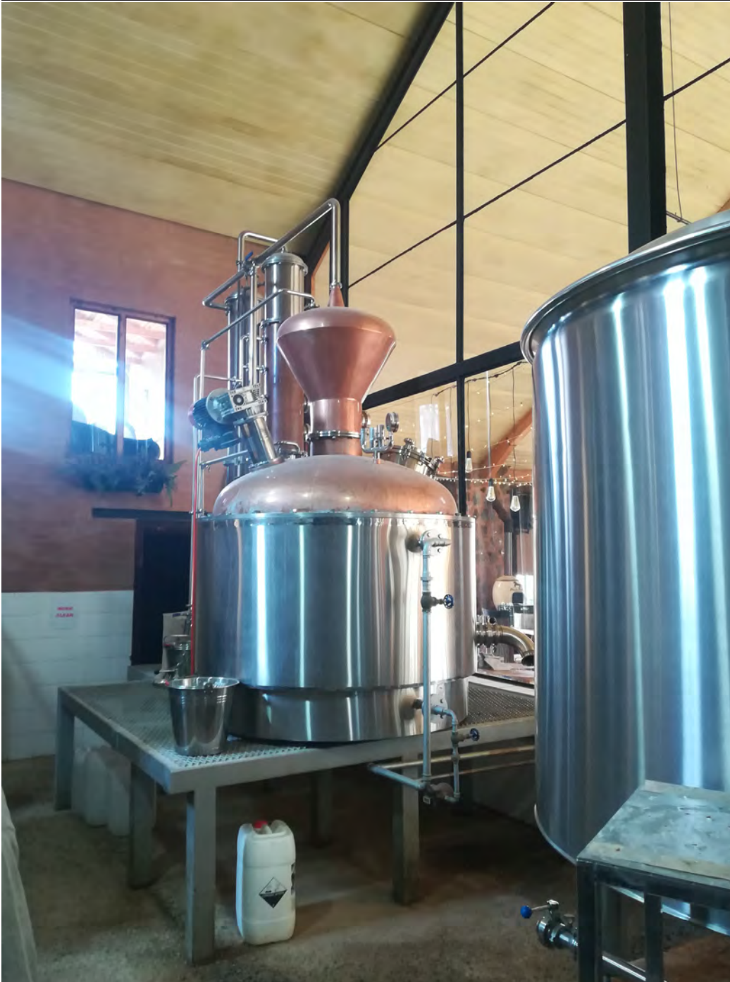
Figure 5.37 - Photograph of the boilers used at Black Horse Distillery; one would notice the copper and stainless steel details used on the boilers to ensure that the flavor infuses with the spirit (Author, 2018).
