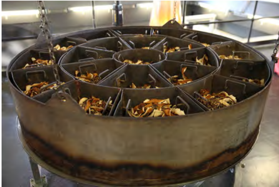
Figure 5.30- Image showing the perforated copper baskets used in the vapor infusion process (Bombay, 2014).
