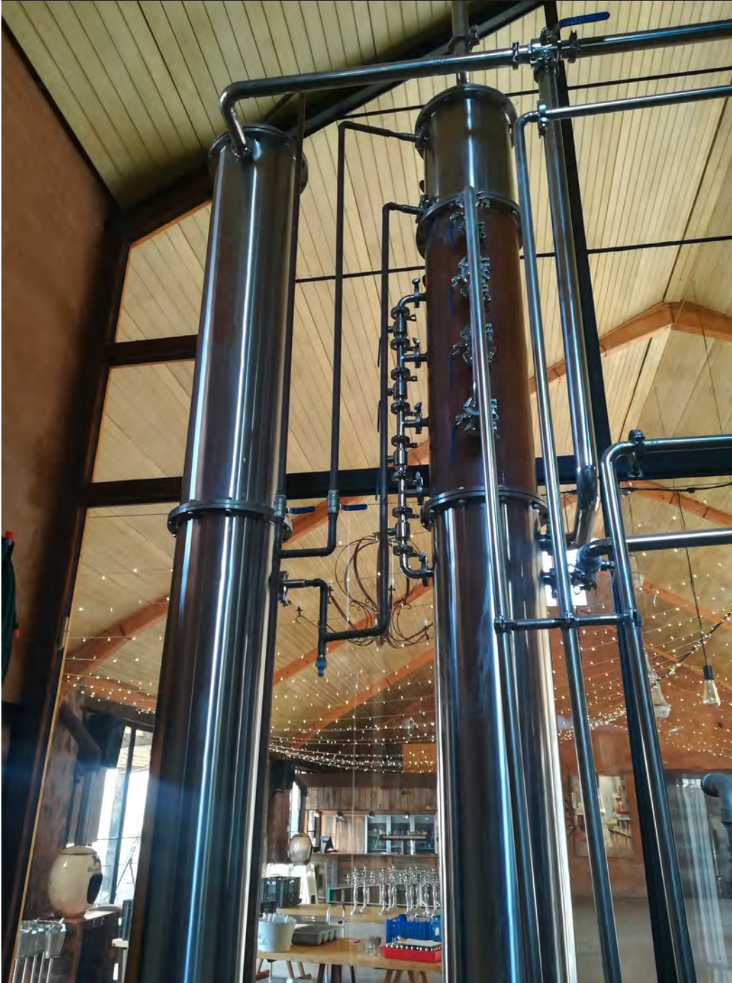
Figure 5.35 - Photograph of the main still that is used for all the brewing and distilling at Black Horse (Author, 2018).
