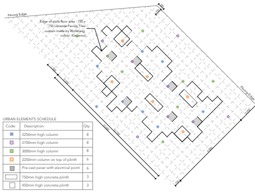
Figure 8.12. Column Position Plan
