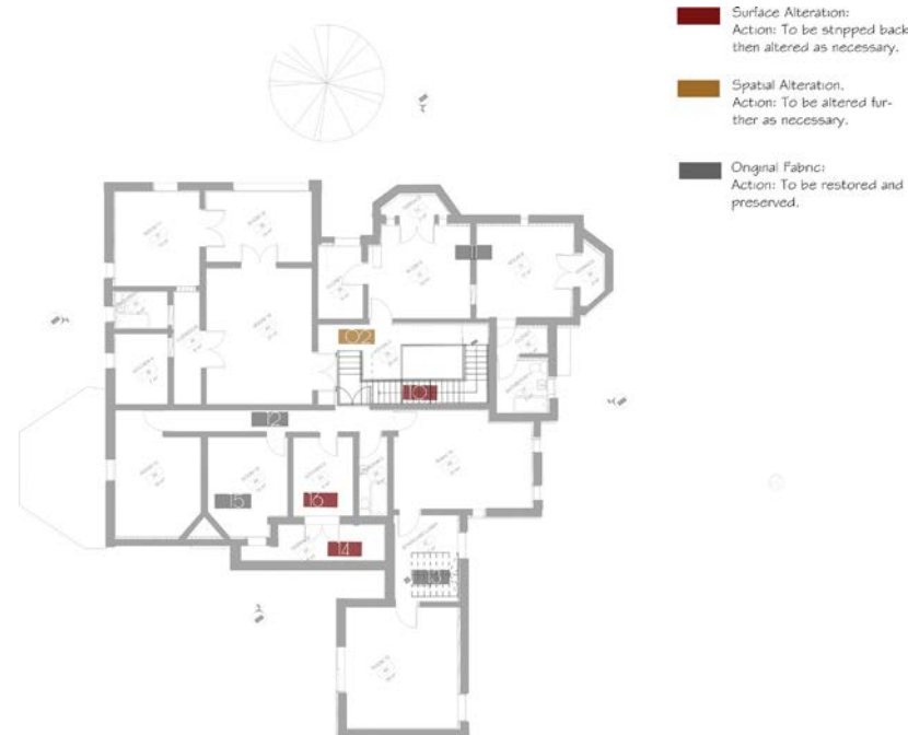
Figure 30: First Floor Interior Analysis (Author 2018)
