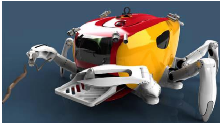
Figure 2.30: Conceptual illustration of CR200 using its front legs as manipulators [39]
