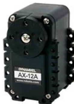
Figure 4.4: Dynamixel AX-12A servo motor used as joint actuators for the PhantomX MK-II [78]
