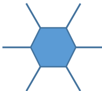
Figure 3.2: Hexagonal, or circular, hexapod body structure, with legs mounted axisymmetrically around body
