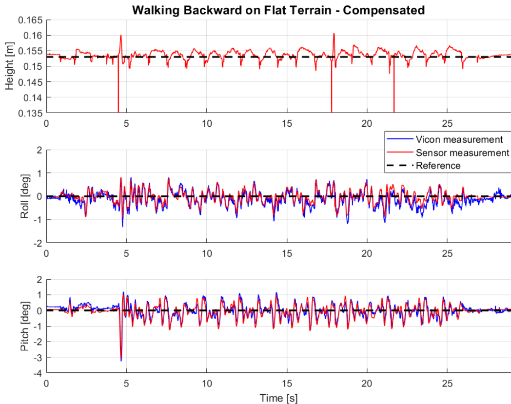
Figure 7.10: Posture response while walking backward on flat terrain, with posture control enabled
