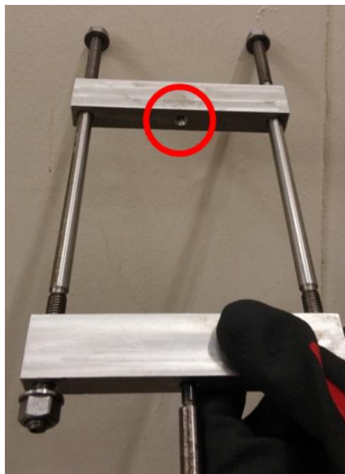
Figure A.4: Underside of cradle bar, showing chamfered hole (circled in red) where cradle is to be rested on force sensor
