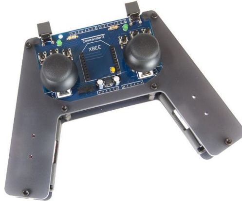
Figure 4.3: ArbotiX Commander – wireless controller for ArbotiX powered walking robots [80]
