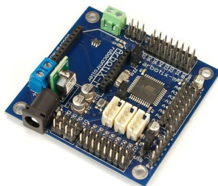
Figure 4.2: ArbotiX-M Robocontroller from Vanadium Labs [79]
