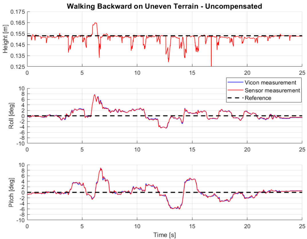
Figure 7.12: Posture response while walking backward on uneven terrain, with posture control disabled
