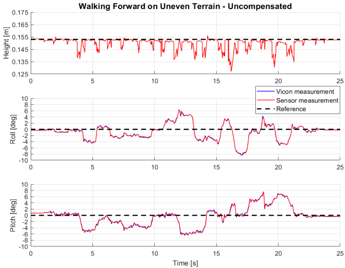
Figure 7.11: Posture response while walking forward on uneven terrain, with posture control disabled
