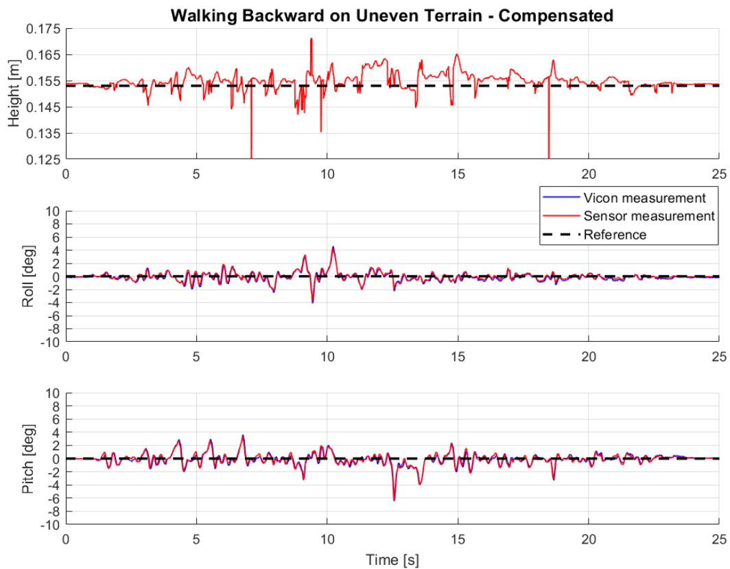
Figure 7.14: Posture response while walking backward on uneven terrain, with posture control enabled
