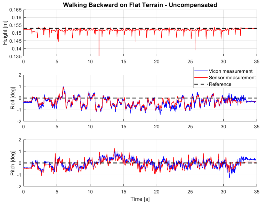
Figure 7.8: Posture response while walking backward on flat terrain, with posture control disabled
