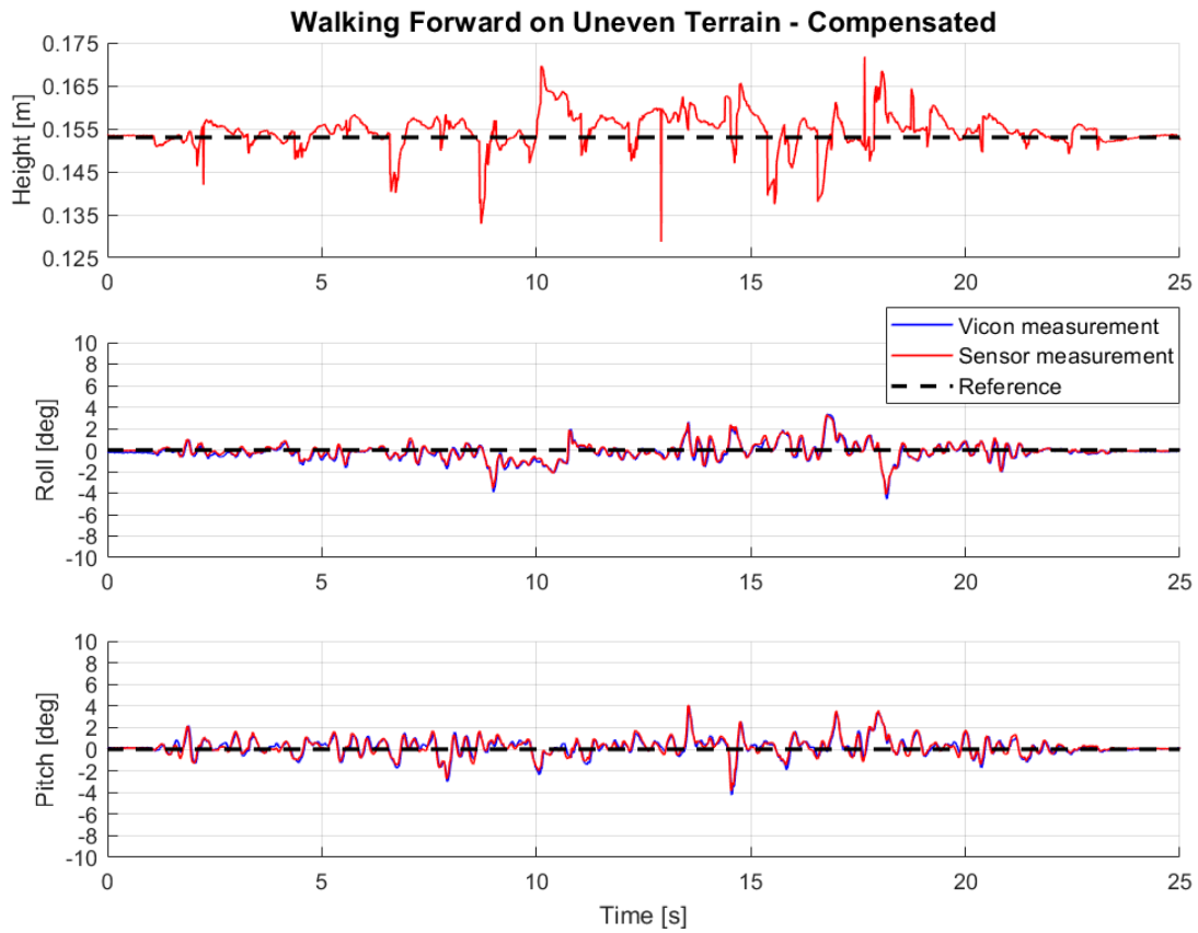
Figure 7.13: Posture response while walking forward on uneven terrain, with posture control enabled
