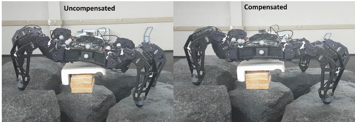
Figure 6.10: Comparison of PhantomX hexapod robot platform standing on uneven terrain, with (right) and without (left) posture control activated [19]
