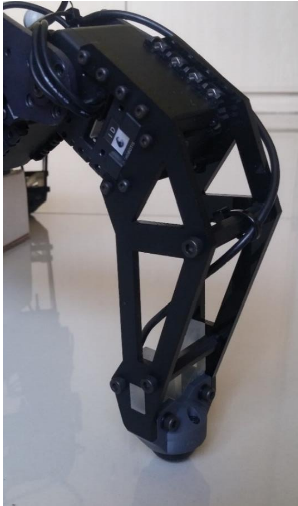
Figure 4.9: Tibia segment of PhantomX with new foot and OptoForce sensor in contact with ground
