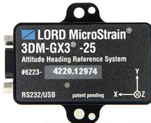
Figure 4.6: LORD MicroStrain® 3DM-GX3® -25 miniature Attitude Heading Reference System [82]
