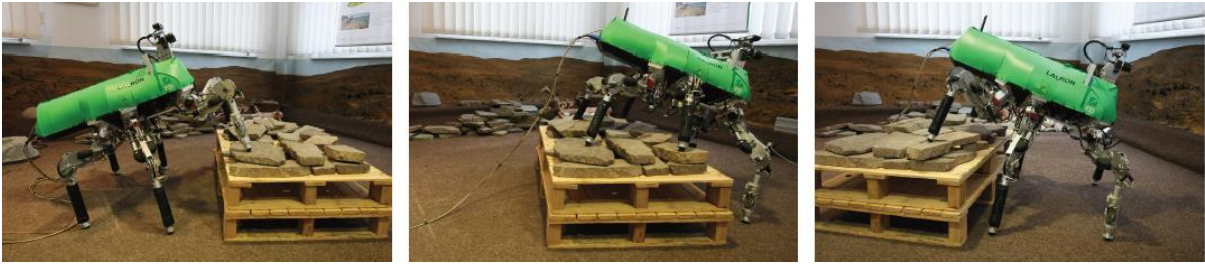
Figure 2.23: Experimental test of LAURON V climbing over obstacle approximately 40 cm high [9]
