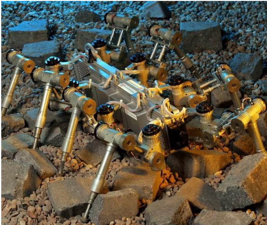
Figure 2.9: SCORPION eight-legged robot designed for space robotics applications [32]
