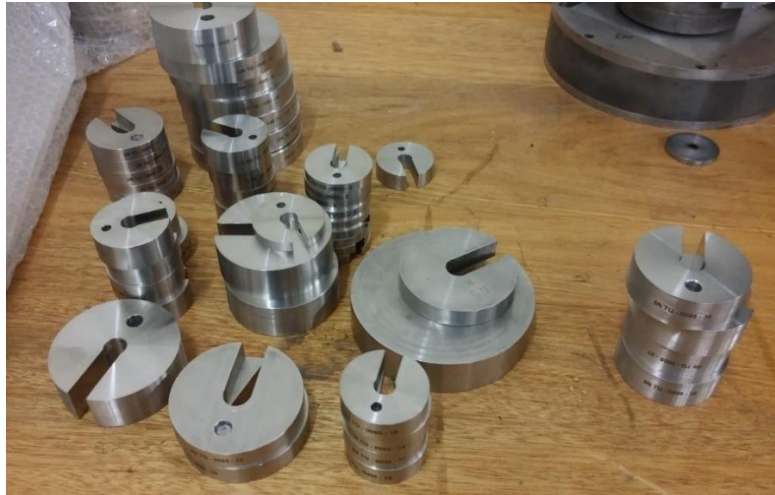
Figure A.1: Weights of various sizes, used for calibration and testing at NMISA's Force Laboratory
