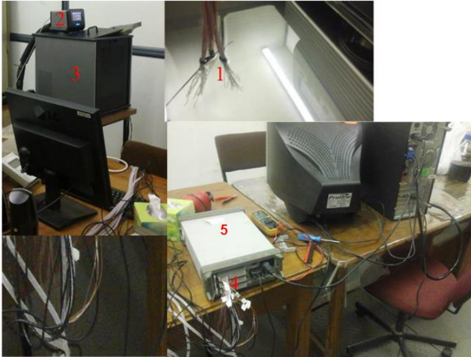
FigureB.1. Thermocouples calibration equipment
