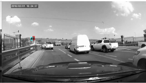
Figure 3.17. Detected traffic lights
