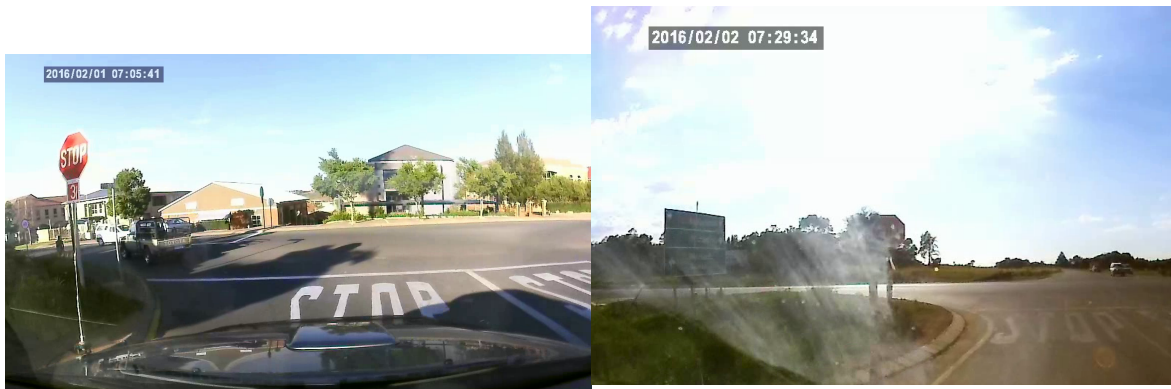
Figure 4.3. Stop sign viewed from a bad angle Figure 4.4. Stop sign viewed through a very dirty wind-screen
