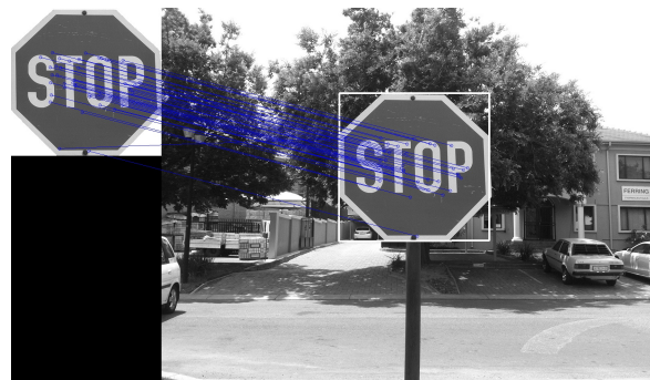
Figure 4.6. Key feature points used by the SURF algorithm
