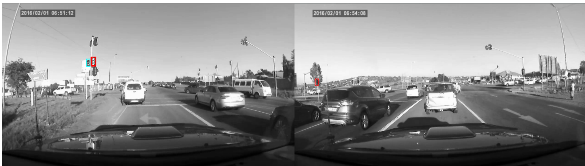
Figure 3.14. Detected traffic lights
