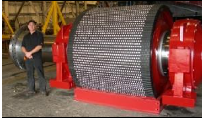
Figure 1.7: Large drive pulley (RAS, n.d.)
