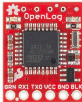
Figure A.0.3: OpenLog microSD card read/writer
