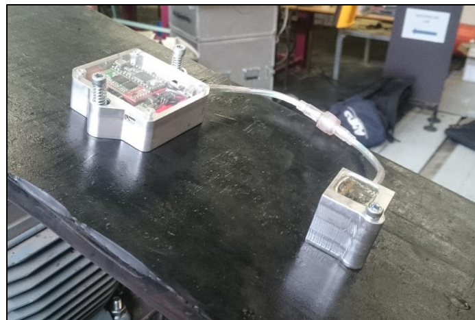
Figure 2.13: Data logger and sensor fixed to the belt
