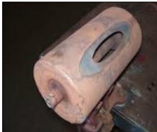
Figure 1.15: Idler seized and belt wore through the steel shell (Intium, 2015)
