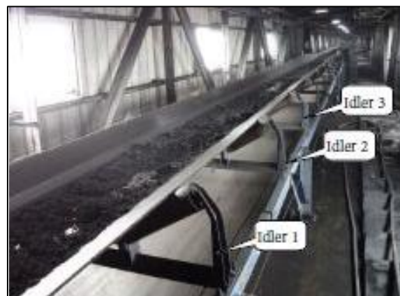
Figure 1.23: Three idlers being monitored by a single accelerometer (Li, et al., 2013)
