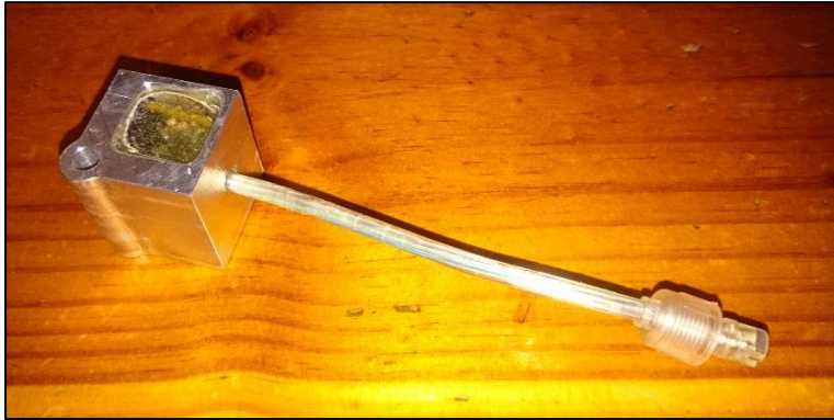
Figure 2.11: LSM6DS33 sensor encased
