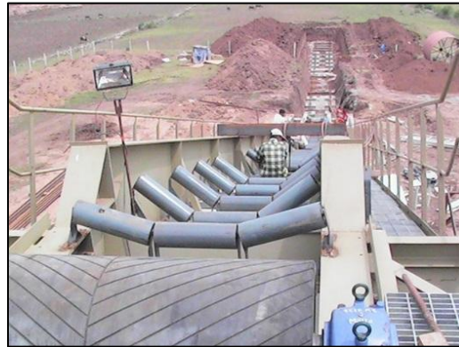
Figure 3.14: Trough made with idlers
