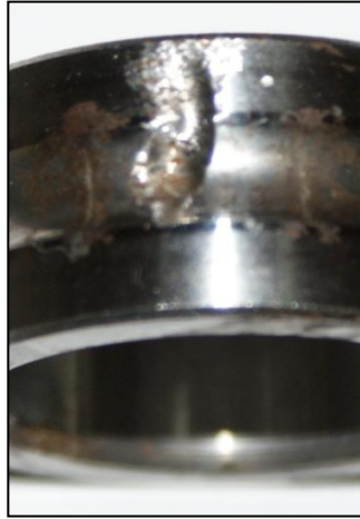
Figure 3.2: Inner raceway defect
