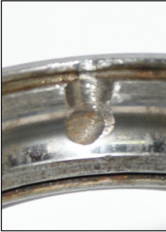
Figure 3.1: Outer raceway defect
