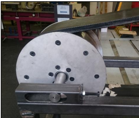
Figure 2.8: Tail pulley and tension/alignment mechanism
