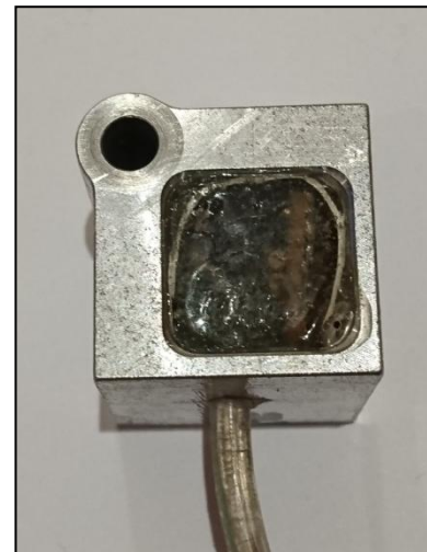
Figure A.0.8: Accelerometer in its aluminium case
