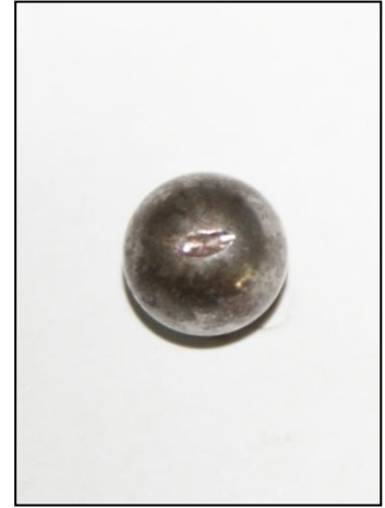
Figure 3.3: Rolling element defect
