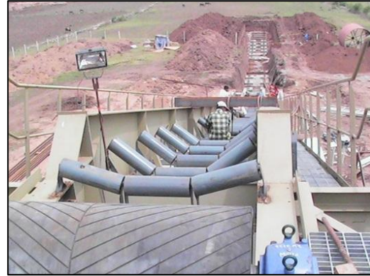
Figure 1.11: Trough created with idlers (Conveytech, 2013)
