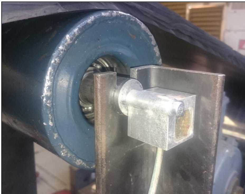
Figure 3.4: Accelerometer attached to idler shaft
