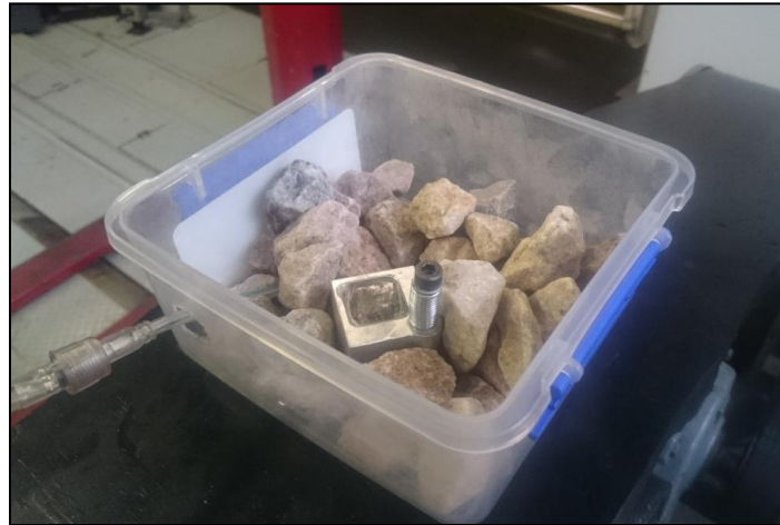
Figure 3.38: Payload surrounding the accelerometer
