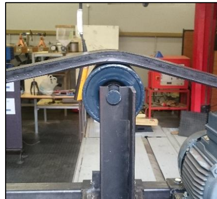
Figure 2.9: Idler and wrapped conveyor belt
