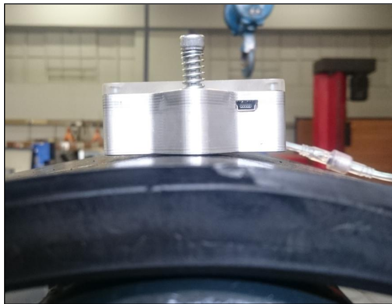
Figure 5.1: Comparison between belt and logger thickness
