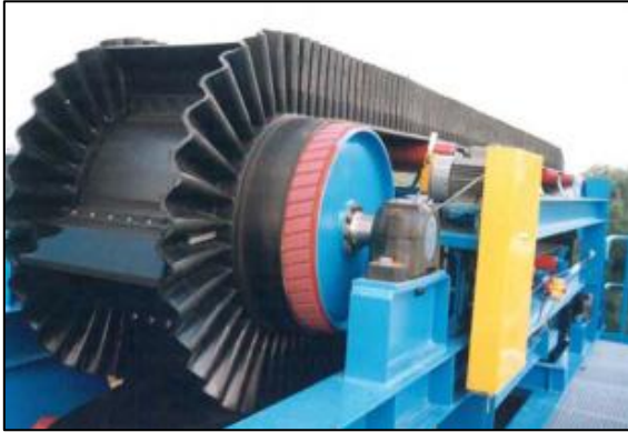
Figure 1.10: Conveyor belt with rubber sidewalls (C.C.Components Pty. Ltd., n.d.)
