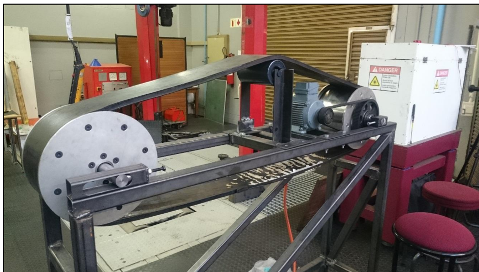
Figure 2.6: Test bench representation of a conveyor
