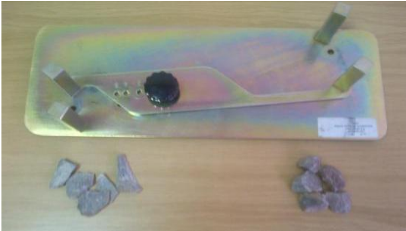
Figure 2.13: Proportional calliper device
