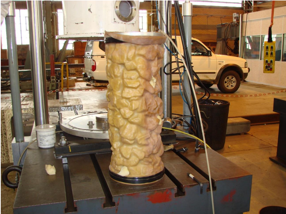
Figure A7: Completed ballast sample
