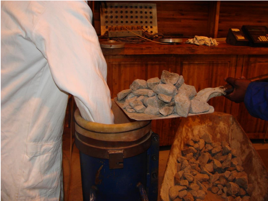
Figure A5: Placement of ballast
