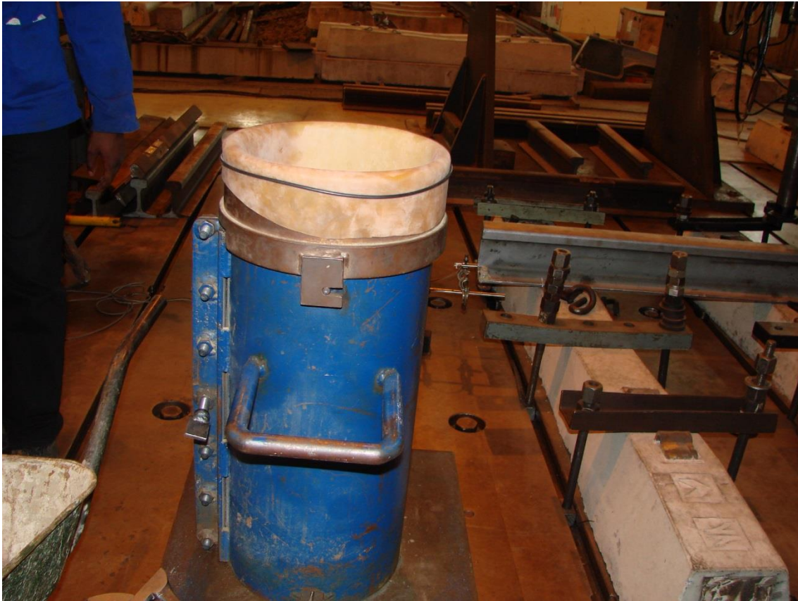
Figure A4: Position of collar, geofabric and membrane
