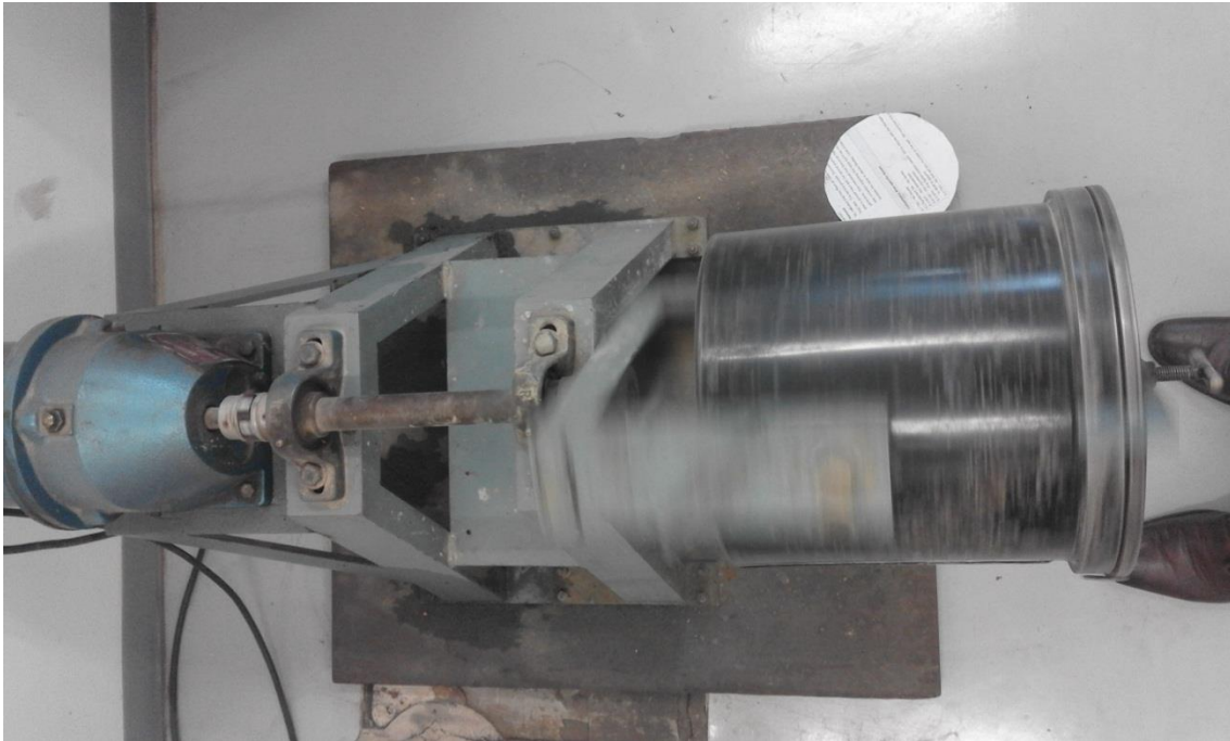
Figure 4.20: Typical Mill Abrasion test machine used for this study
