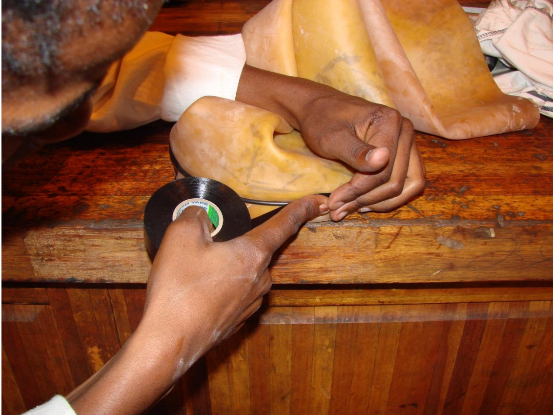
Figure A1: Attaching membrane to baseplate
