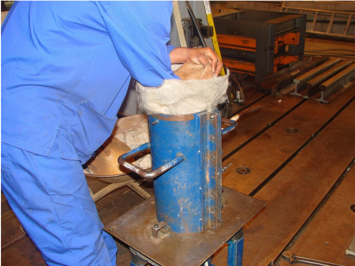
Figure A3: Placing of the geofabric
