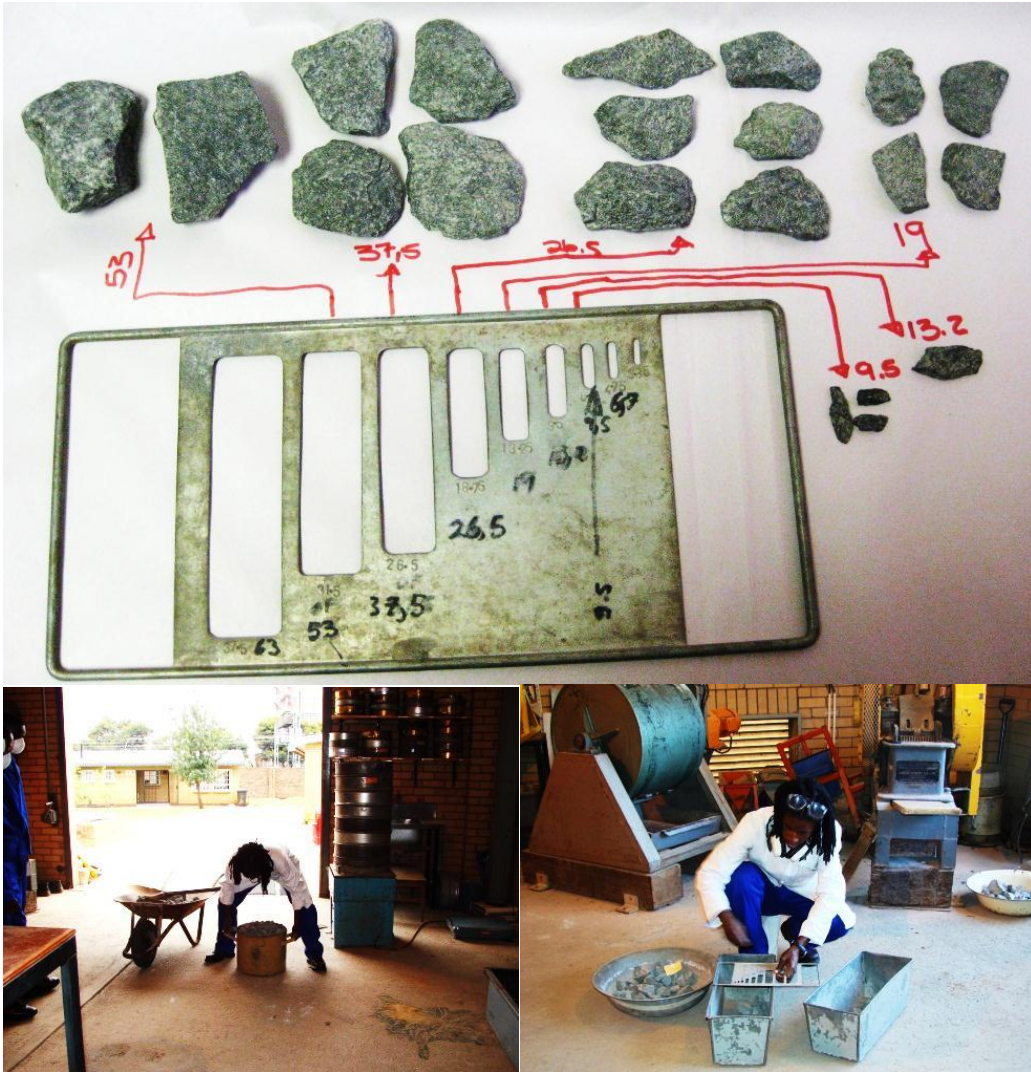
Figure 2.12: Current test method using a flat gauge (Courtesy of TFR)
