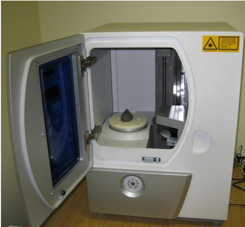
Figure 2.4: 3D-laser scanning set-up at CSIR
