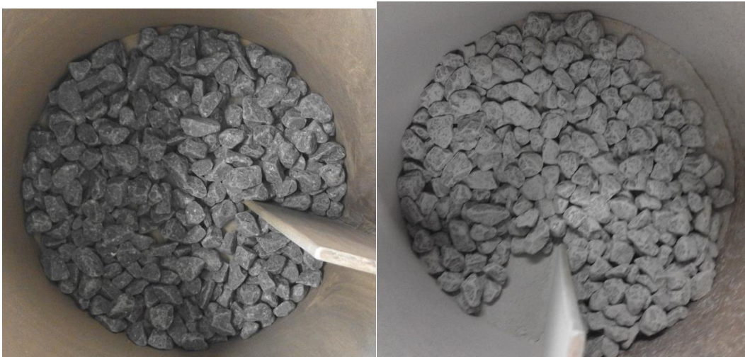
Figure 4.21: Ballast sample before and after a Mill Abrasion test
