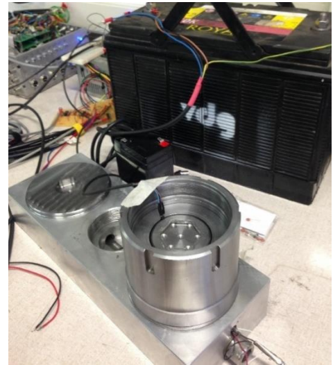
Figure 4. 11: Experimental characterisation of the assembled MR valve
