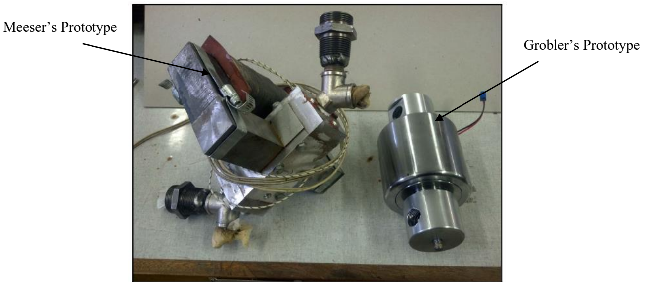
Figure 2. 6: Grobler's first prototype MR valve (Right) compared to Meeser's MR valve (Left). (Grobler 2016)
