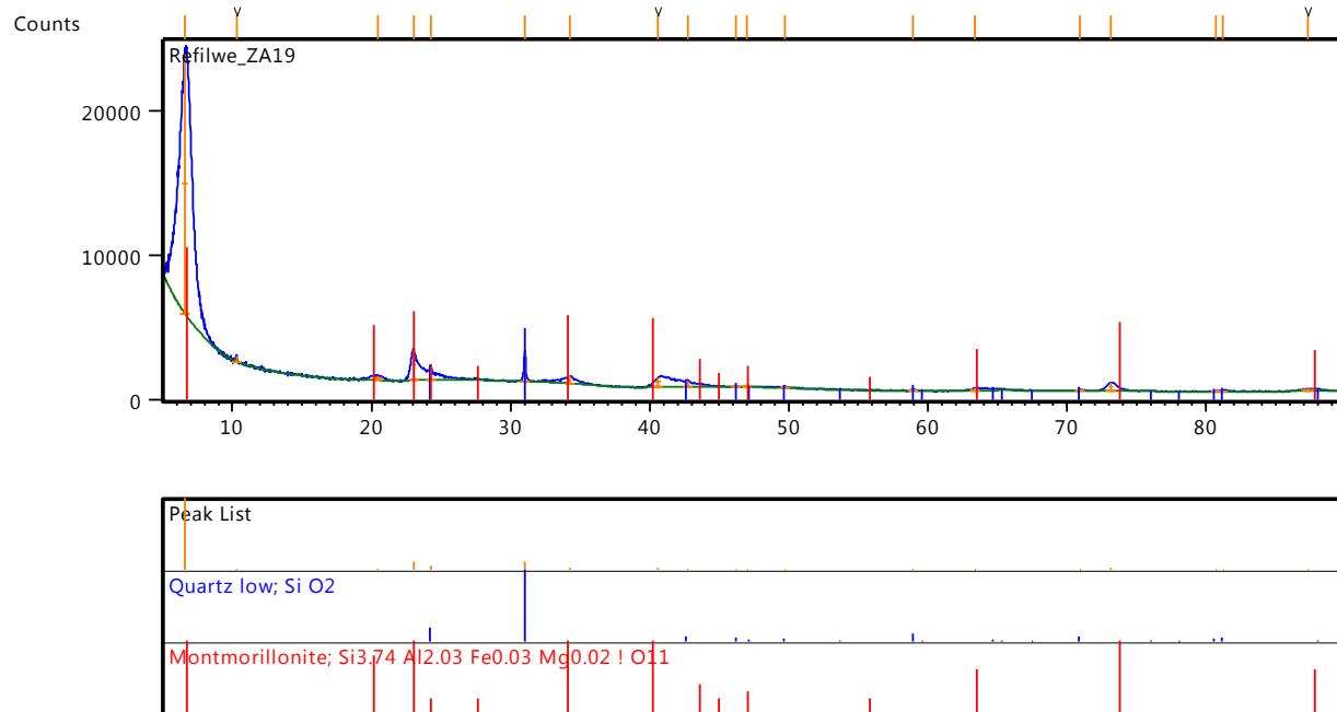
2017.07.04 The sample was prepared according to the standardized Panalytical backloading system, which provides nearly random distribution of the particles.
