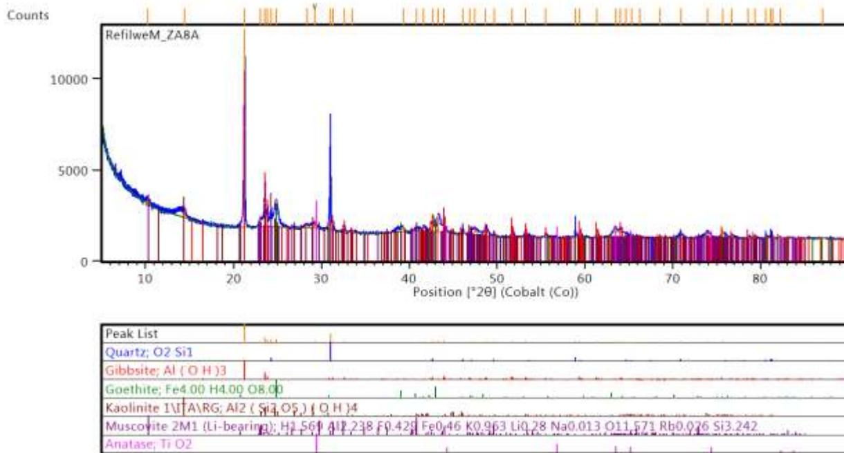
2015.02.19 The samples were milled in a tungsten carbide vessel and prepared according to the standardized Panalytical backloading system, which provides nearly random distribution of the particles.
