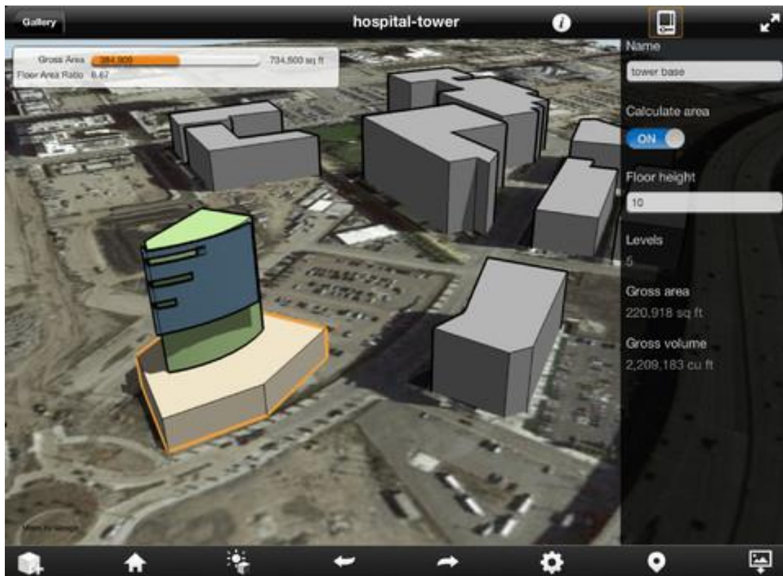
Figure 6.33. The user interface within Autodesk Formit®, representing BIM-based CAD for real-time geometric analysis, and early concept formulation Source: https://aec-apps.com/sites/default/files/mzl.pjjgupy.480x480-75_0.jpg [Viewed 10 June 2016]
