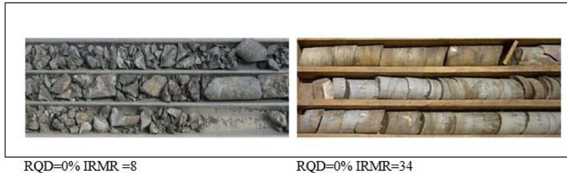
Figure 2-4 Problems with RQD and classification systems that include RQD (Jakubec 2013)
