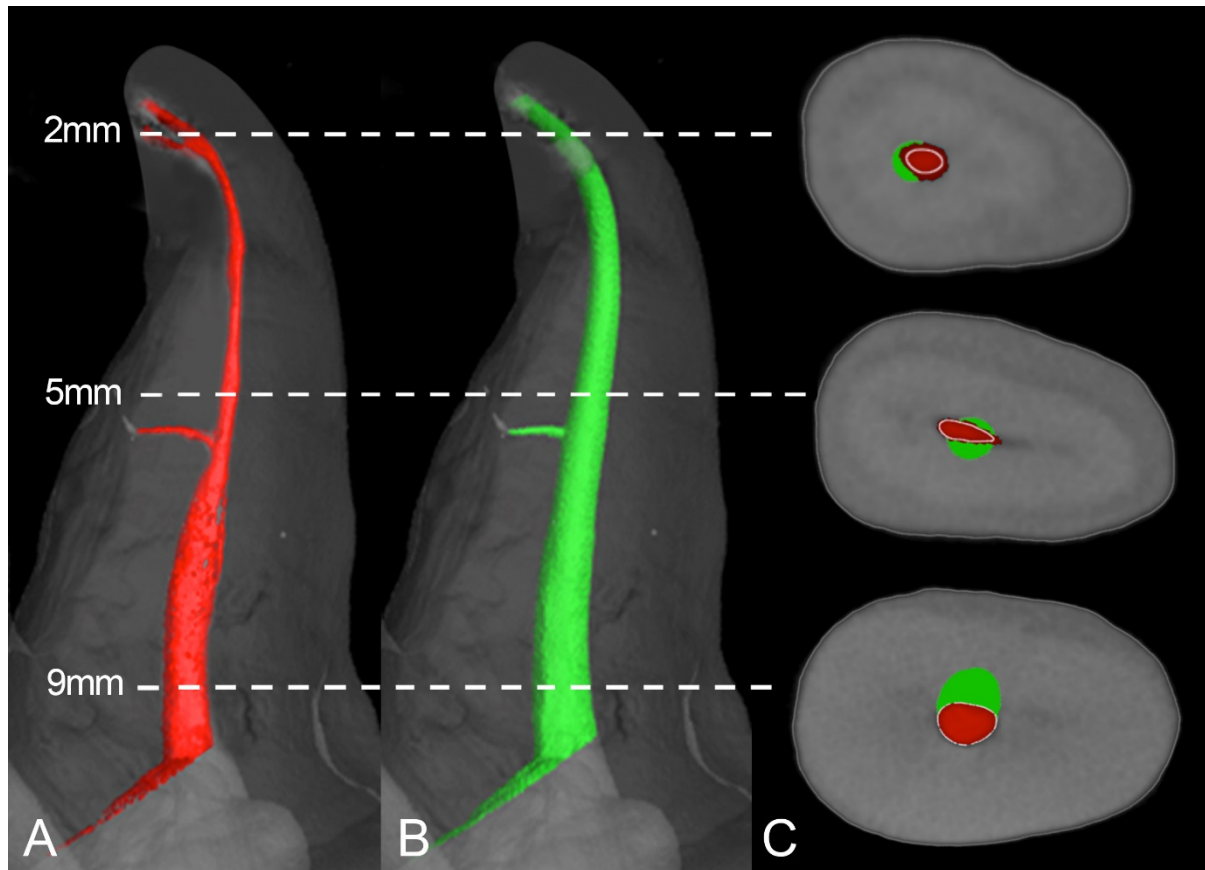
Figure 4.41: A representative sample of 3D images of a mesio-buccal root canal system: (a) pre-operative uninstrumented canal volume (red); (b) canal volume after canal preparation with the OneShape instrument (green); (c) the superimposition of the canal systems and the changes of the canal axis before (red) and after canal preparation (green) with the OneShape instrument at the apical-, midroot-, and coronal levels
