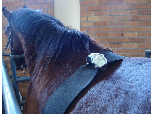
Figure 2. Heart rate monitor and heart rate monitor belt attached by means of a surcingle.
