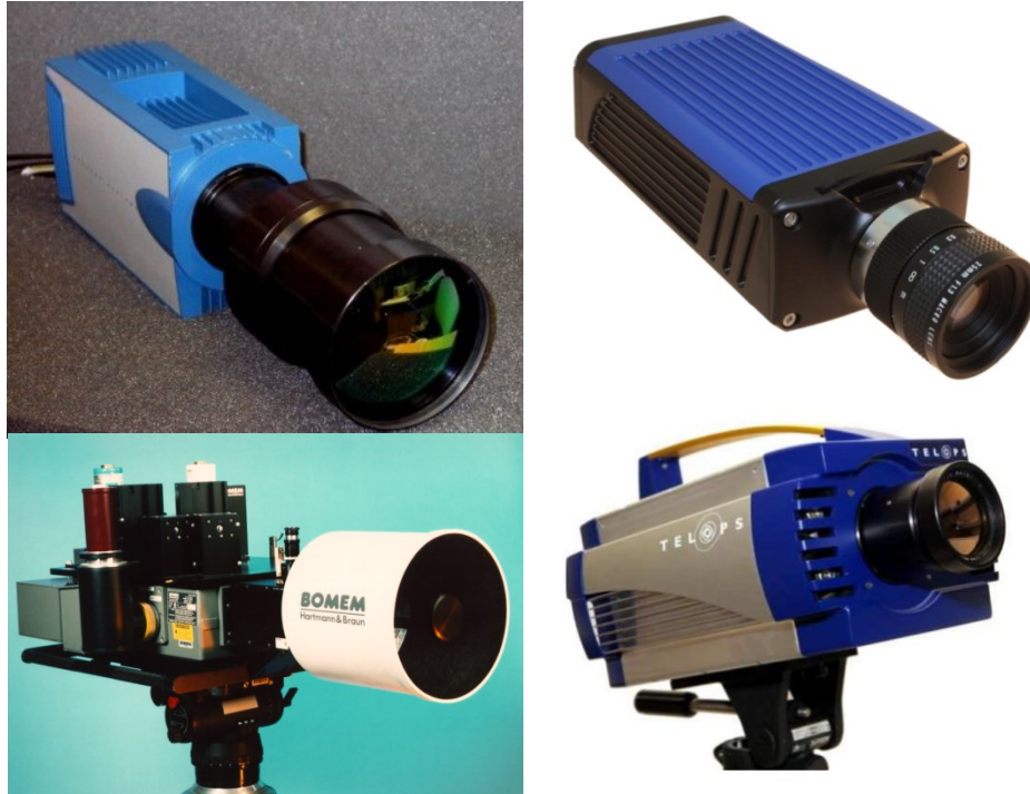
Figure 2-2 Clockwise from top left: Cedip Jade III MWIR camera, FLIR SC2500 SWIR camera, Telops TEL-1000-VLW camera, Bomem MR200 spectroradiometer.
