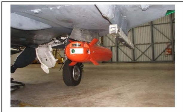
Figure 1. The pod containing the backward facing MWIR camera. This camera is directed towards the target aircraft through the circular Si window. The rectangular perspex window above the Si window allows a visual camera to be installed for the purpose of reference recordings.
