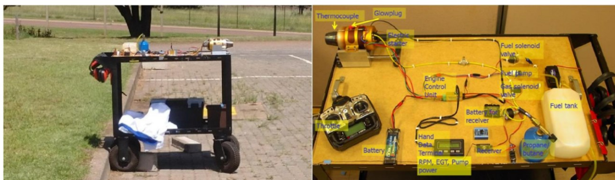
Figure 2. Micro turbine set-up used for IR measurements. The turbine used a propane/butane gas mixture only for startup, after which the fuel supply was switched to Jet A-1 fuel.
