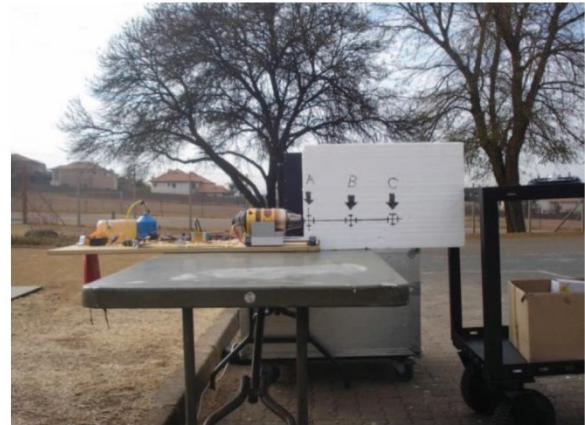
Fig. 7. Close-up of mask used as reference to adjust three FOV positions of SR in small FOV session.
