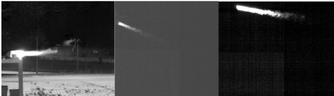
Figure 5. MWIR recordings of the micro turbine engine running at 135 000 RPM (left), rear end of aircraft at full thrust (middle) and aircraft at full thrust with afterburner (right).
