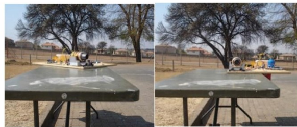
Fig. 4. View from MWIR camera position for AAs of 135° (left) and 180° (right) as used in AA scan session.
