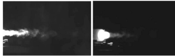
Fig. 13. Plume recording in MWIR band for 90^\circ (left) and for 135^\circ (right) AAs, both for 145 000 RPM, where no filter was used to have plume radiance well above detector noise level.
