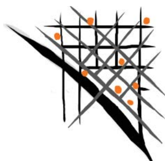
Figure 98. By introducing a rotated grid, the sensibility of the orthogonal grid can be maintained as well as creating the opportunity to connect the dispersed nodes with legible more direct axes. Thus the area begins to favour pedestrian comfort and ease of access.
