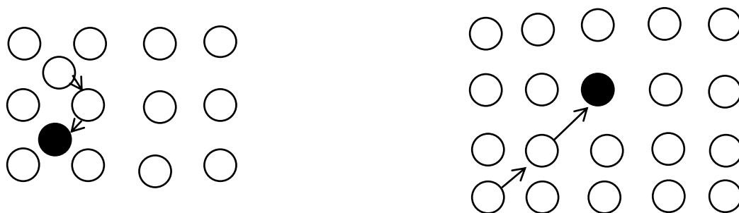
Figure 2-3: The interstitialcy mechanism, (a) before and (b) after interstitialcy diffusion.
