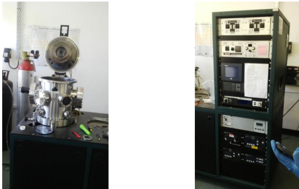
Figure 6-3: Images of AJA Inc. Orion 5 sputtering system at the University of Zululand.
