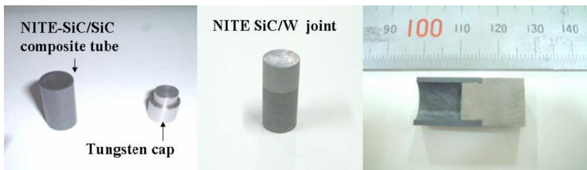
Figure 1-5: Joint of Nano-powder Infiltration and Transition Eutectoid (NITE)-SiC/SiC composite tube and tungsten cap on the fuel pin taken from [51].
