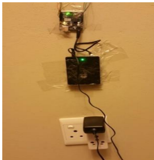
Figure 4.8. Shows the modified power source, power to the microcontroller is routed through a power bank.
