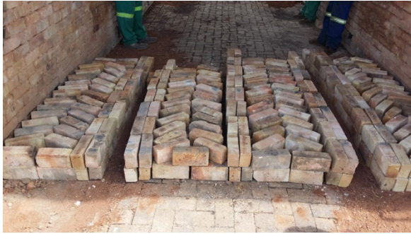
Figure 84: First and second course of bricks packed from one end of the kiln to the middle (left); and from the other end to the middle of the kiln (right)
