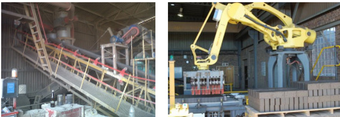
Figure 19: Crusher conveyor at Bert's Bricks (left) and robotic arm at Nova Bricks (right) South Africa
