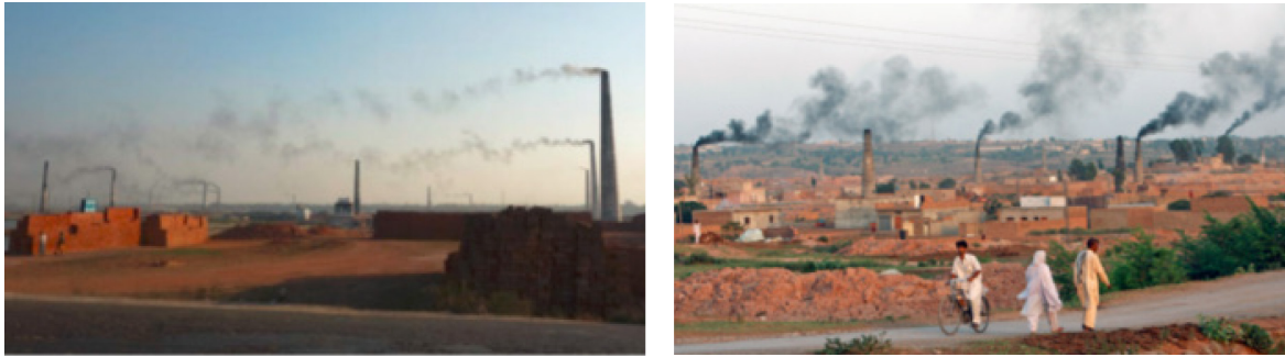
Figure 15: Clusters of fixed chimney BTK operating in Dhaka (left) and Pakistan (right) (Guttikunda & Khaliqzaman, 2014; Schmidt, 2013)
