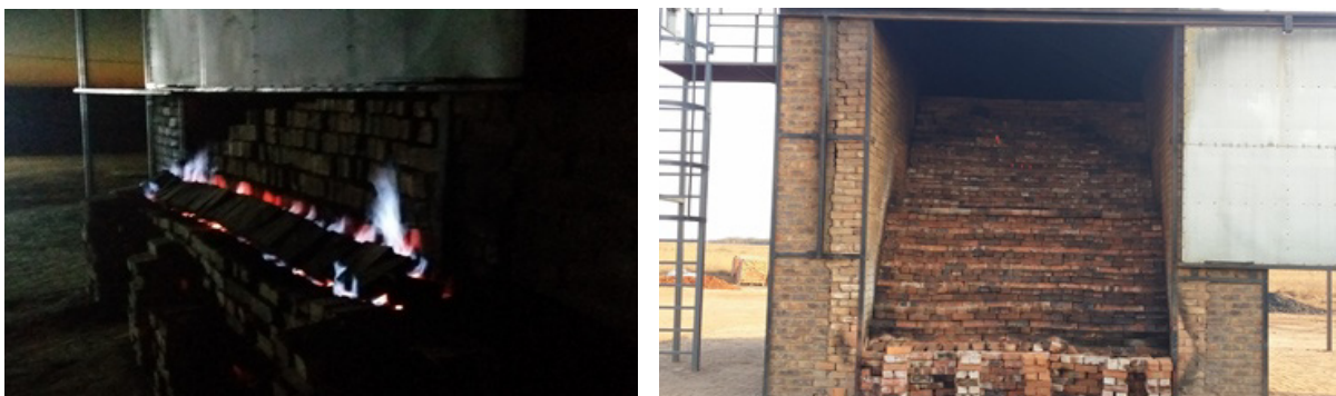
Figure 43: Model kiln scintille ablaze during night-time (left); inner chamber of model kiln at advanced stage of firing during day-time with side boards opened to take photograph (right)
