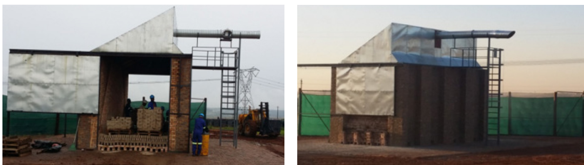
Figure 32: On-going model kiln packing process (left); packed model kiln with sliding doors closed (right); – note position of extraction duct and sampling platform and green mesh windscreen
