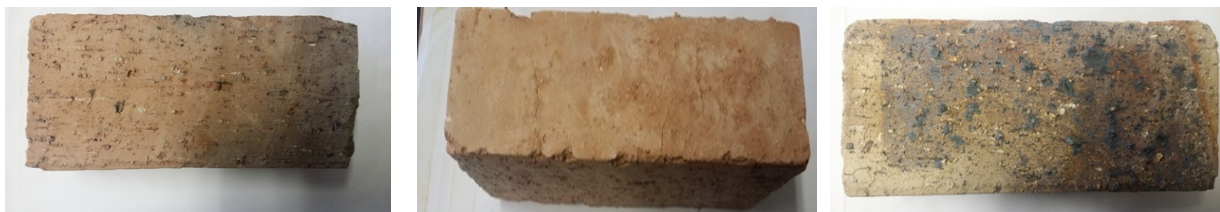
Figure 87: Under-fired brick (left), partially fired brick (middle) and evenly fired brick (right) from the propane gas firing run
