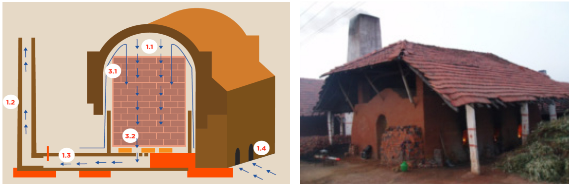
Figure 11: Schematic (left) and structure (right) of a typical DDK (Maithel et al , 2014b; Pradhan, 2015)
