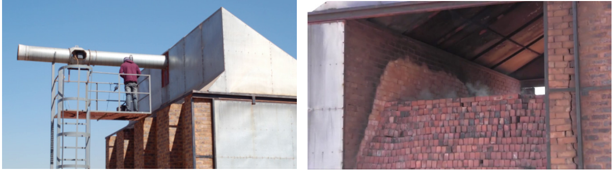
Figure 44: On-going stack monitoring at model kiln (left); visible smoke emitted from the bricks towards the roof duct while side boards are opened to take photograph (right)
