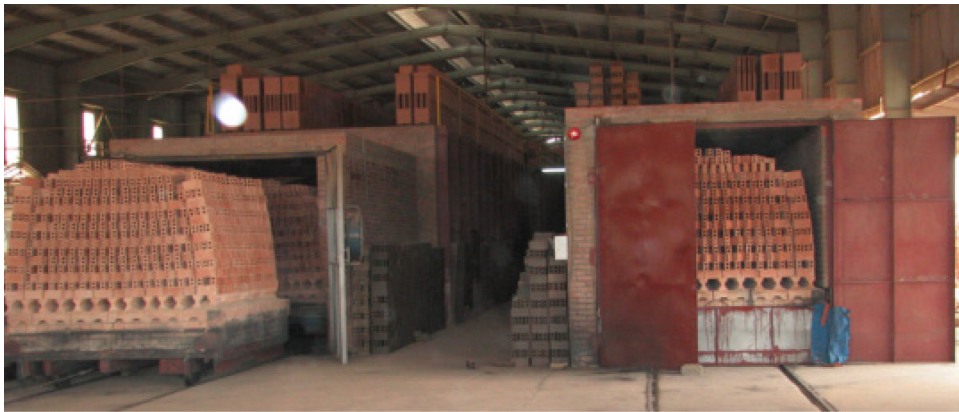
Figure 6: Inner chamber of a tunnel kiln (Maithel et al , 2014h)
