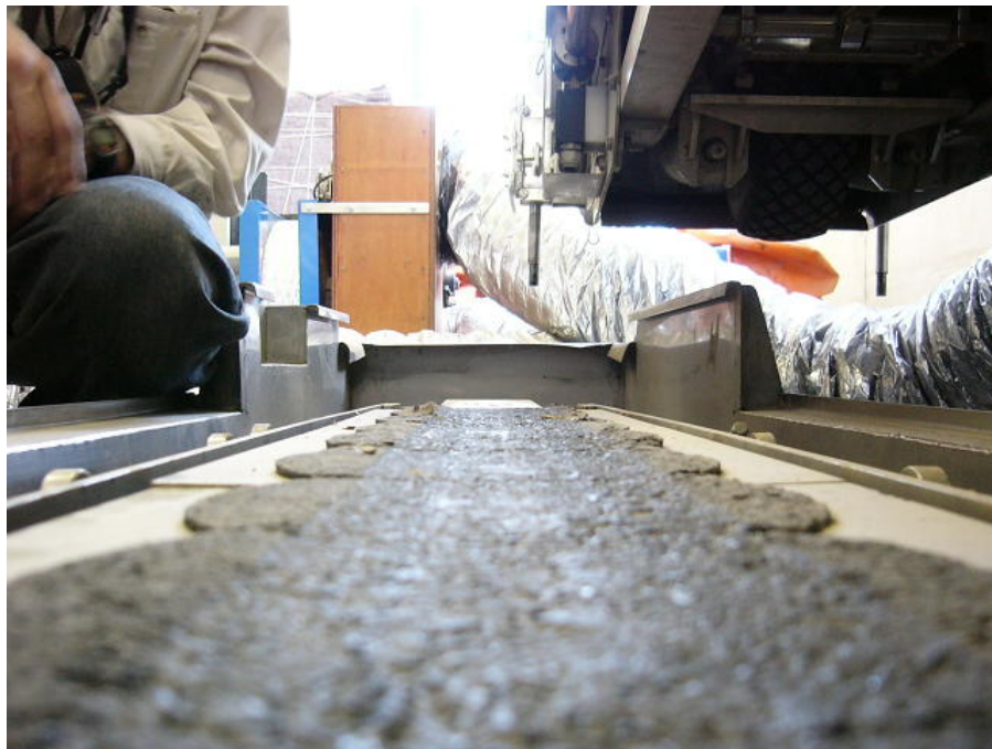
Figure 1: Briquettes after 100 000 MMLS3 test axle loads.
