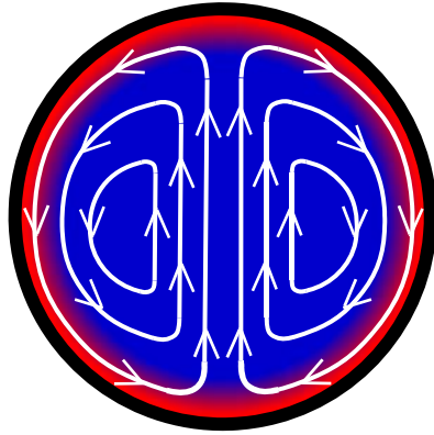
Fig. 2.1: Schematic representation of the counter-rotating vortices caused by free convection effects.
