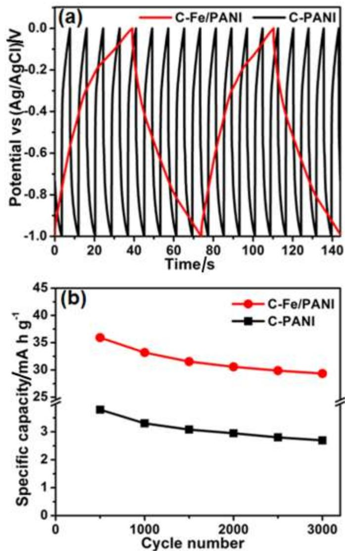
**Figure S3.** (a) GCD curves of both C-Fe/PANI and C-PANI at 5 A g<sup>-1</sup>. (b) The specific capacity of both C-PANI and C-Fe/PANI as a function of a cycle number at a current density of 5 A g<sup>-1</sup>.
