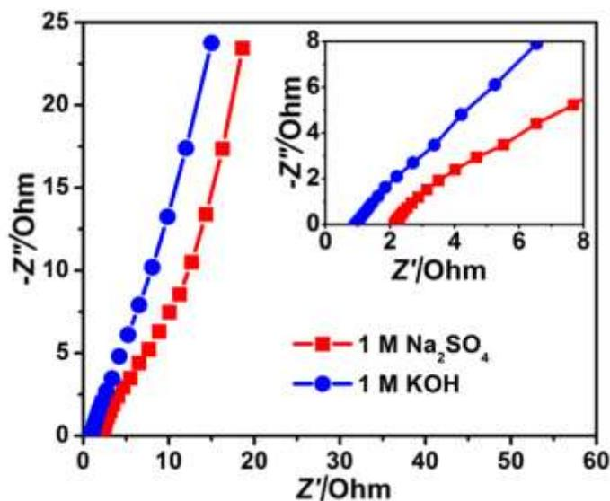
**Figure S2.** The Nyquist plots for  $\text{VS}_2$  in different electrolytes. The inset shows the enlarged high-frequency region of the plot.
