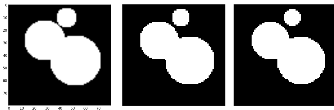
(a) Original image f to be eroded (b) Erosion of f by elementary cross (c) Erosion of f by elementary square
