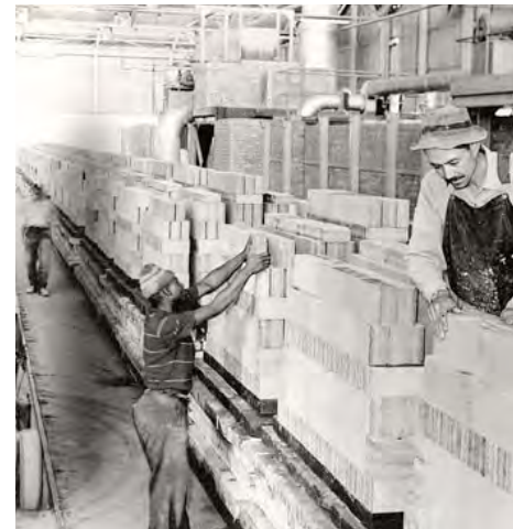
Fig. 3.3. & 3.4. Two historic photographs of workers sorting through raw materials extracted from site and stacking fire bricks manufactured in the Vereeniging Brick & Tile warehouse ( http://www.verref.co.za/index.php?page=gallery-history accessed 10 April 2017).
