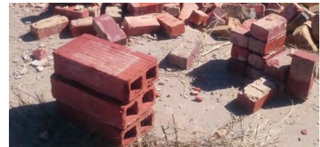
Fig. 8.10. bottom: 220 x 110 x 75 mm porous firebricks found on site (Author, 2017).
